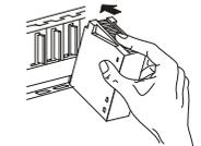
② Push the module in the direction of the arrow to load it into the base unit.
