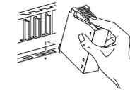
① After switching off the power supply, insert the module fixing latch into the module fixing hole of the base unit.
