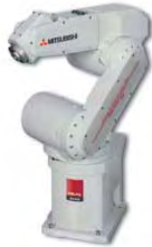
Articulated arm robots are equipped with internal cable connectors and compressed air supplies.
