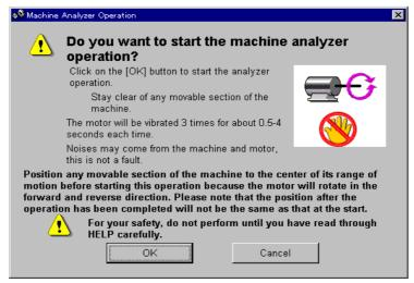
Machine analyzer operation start screen
