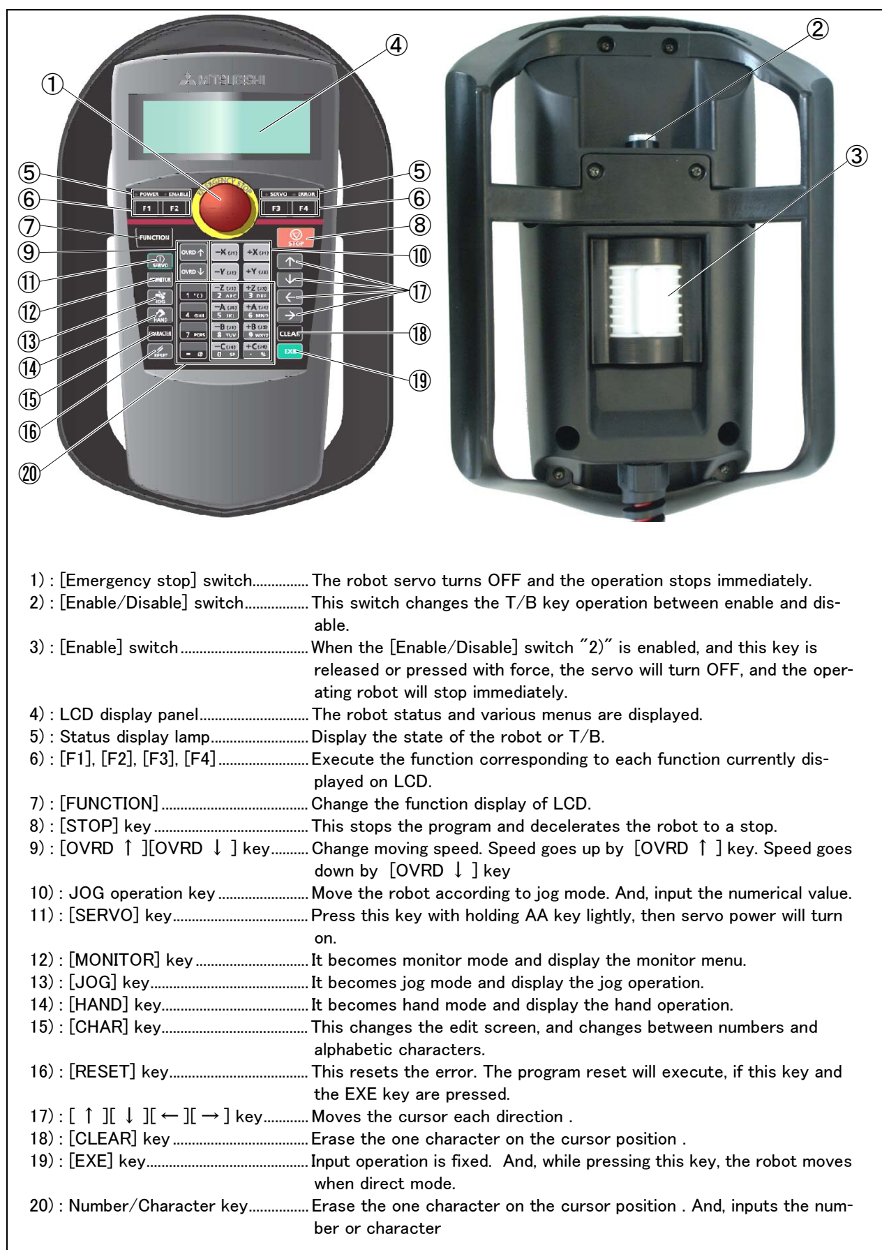
Fig.3-27 : Teaching pendant key layout and main functions
