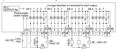
Terminal blocks are not equipped with built-in fuses. In order to prevent breakdown of circuits caused by load short-circuit, provide a fuse of 5 to 10 A for every four points.
