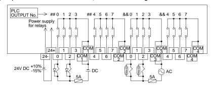
Terminal blocks are not equipped with built-in fuses. In order to prevent breakdown of circuits caused by load short-circuit, provide a fuse of 5 to 10 A for every four points.
