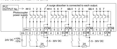
Terminal blocks are not equipped with built-in fuses. In order to prevent breakdown of circuits caused by load short-circuit, provide a fuse of 2 A for every four points.
