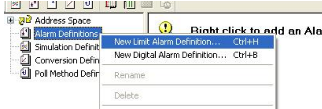
Creating a New Limit Alarm Definition
