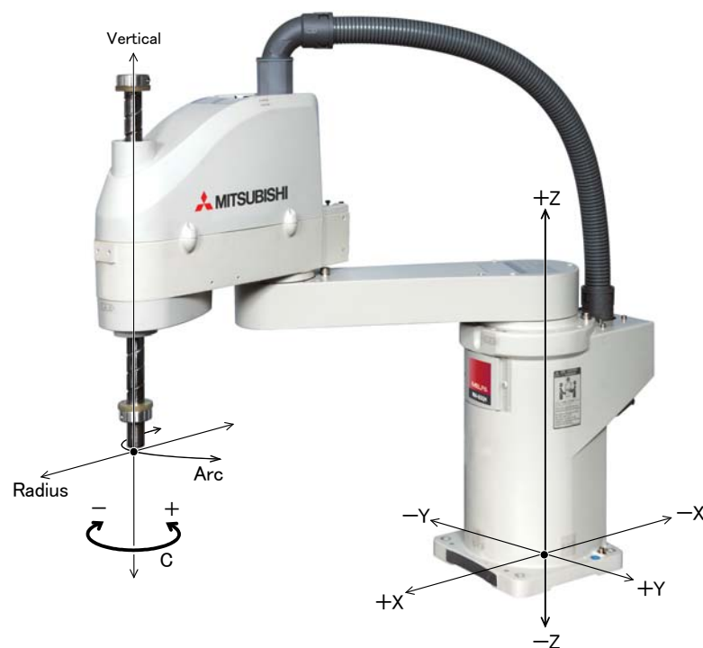
Fig.2-19 : 3-axis XYZ jog operation
