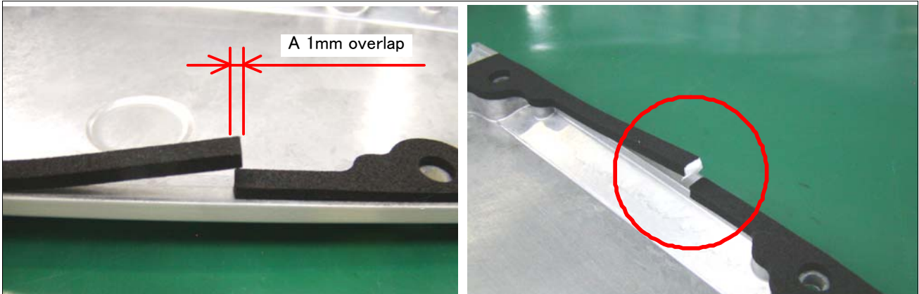
[1] Cut the packing so that there is a 1mm overlap at the end.
