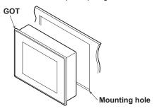
(2) Place the mounting fixtures (included with GOT) on the mounting fixture attaching part of the GOT, and fix them by tightening the mounting screws in the torque range of 0.36 to 0.48NÅEm. (Failure to do so may distort the panel and make a surface waviness on the protective sheet.)
