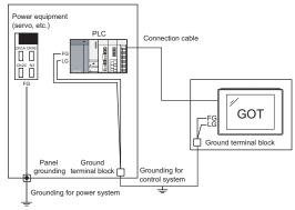
\* Ground the control system, especially modules communicating each other, to one end.
