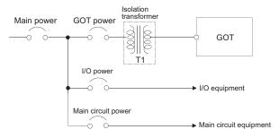
Wiring diagram for power supply
