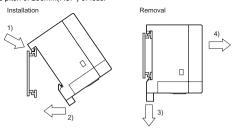
Applicable DIN rail [TH35-7.5Fe and TH35-7.5Al (conforming to JIS C2812)]
