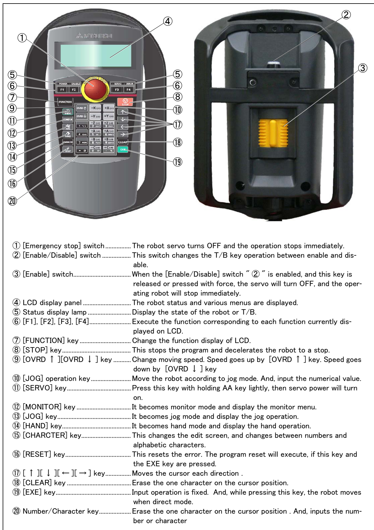
Fig.3-22 : Teaching pendant key layout and main functions
