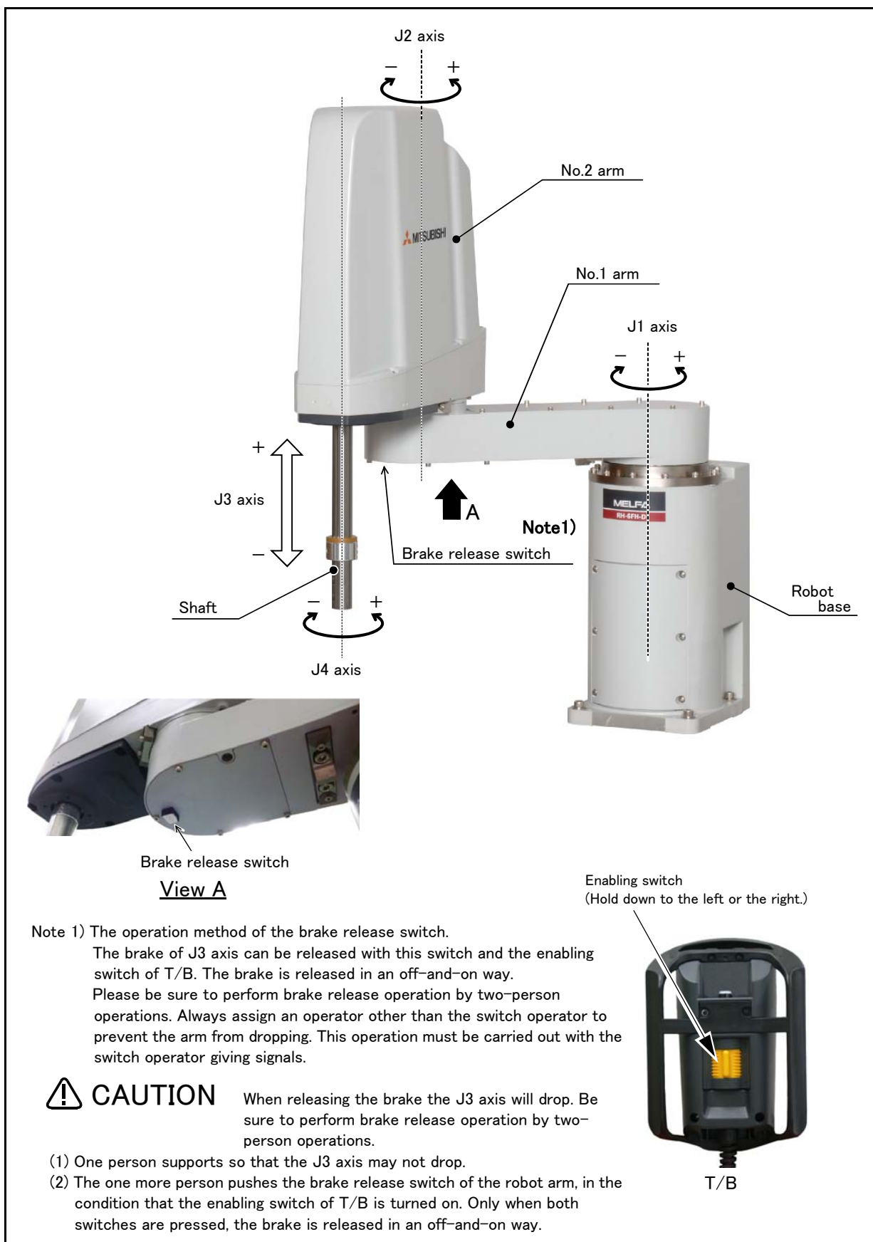
Fig.2-11 : Names of each part of the robot
