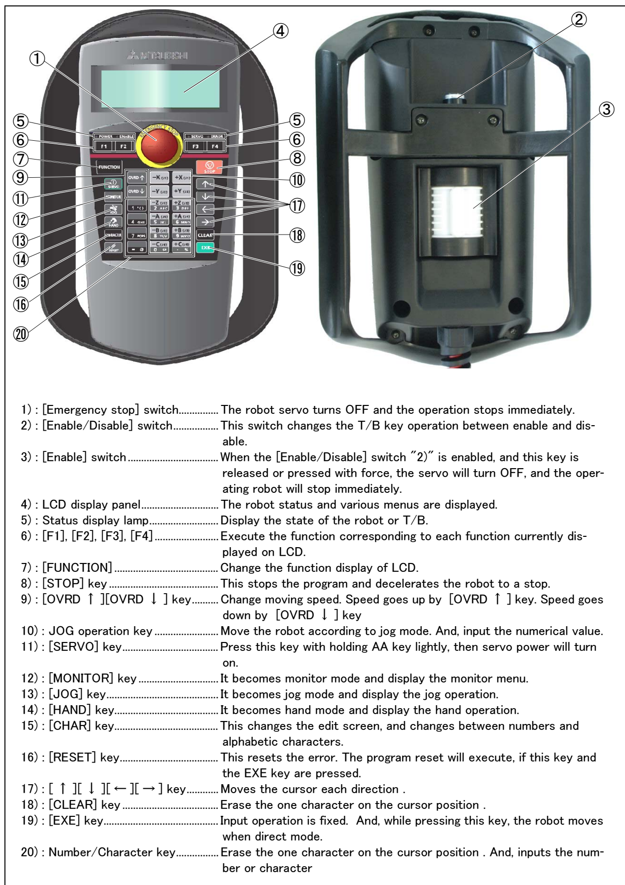
Fig.3-34 : Teaching pendant key layout and main functions
