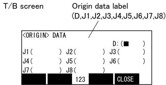
Fig.2-15 : Correspondence of origin data label and axis
