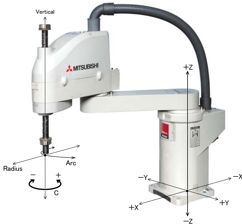
Fig.2-19 : 3-axis XYZ jog operation
