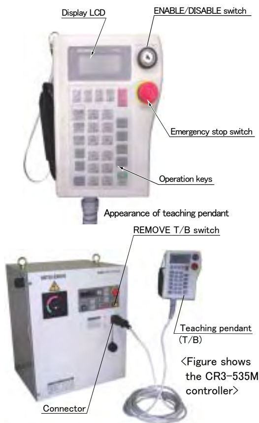
Fig.2-7 : Installing the T/B (control power OFF)
