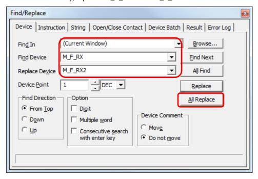
By performing the steps above, the CC-Link IE field master/local FB can be used for the second module.
