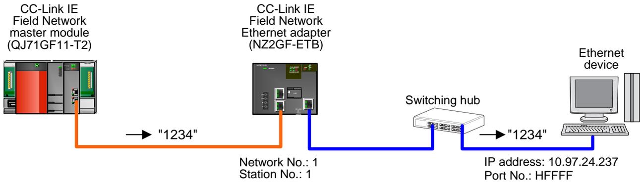
The CC-Link IE Field Network master module sends on-demand data to the Ethernet device connected to an Ethernet adapter with the following conditions.
