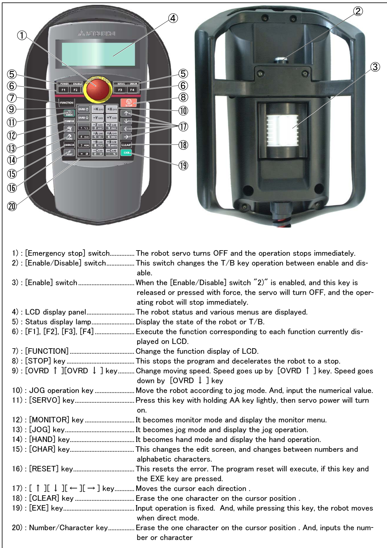
Fig.3-32 : Teaching pendant key layout and main functions
