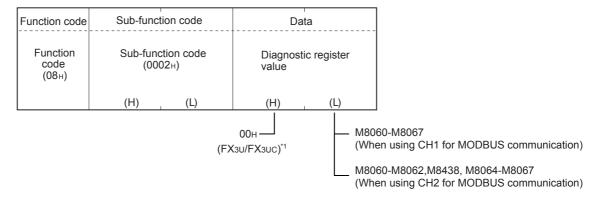
\*1. When using 3rd party products. The high byte (H) does not equal 00H. For further information on the specifications for the slave refer to Chapter 9.
