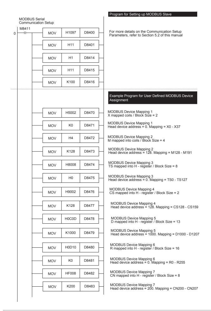
The following tables provide the values for MODBUS address allocation for Bit devices and word devices for the example stated above:
