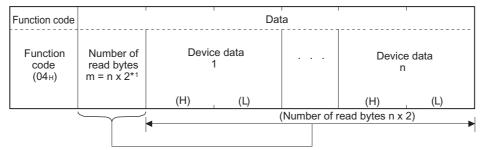
\*1 For example, if n = 4, the number of bytes is calculated as 4 x 2 = 8 bytes
