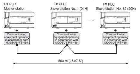
MODBUS Slave Nodes do not need to be numbered in any specific order.
