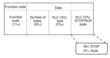
The slave (FX-Series MODBUS Communication ADP) will return 'F3' as the PLC CPU type data to the Master:
