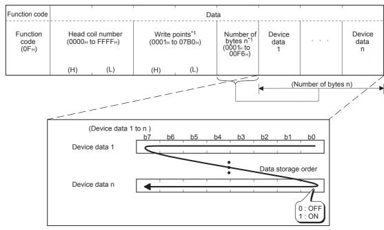
The values (ON/OFF) stored into the device data 1 to n are written to the coils in order from low-order to high-order bits of the device data.
