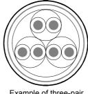
Example of three-pair cable structural drawing
