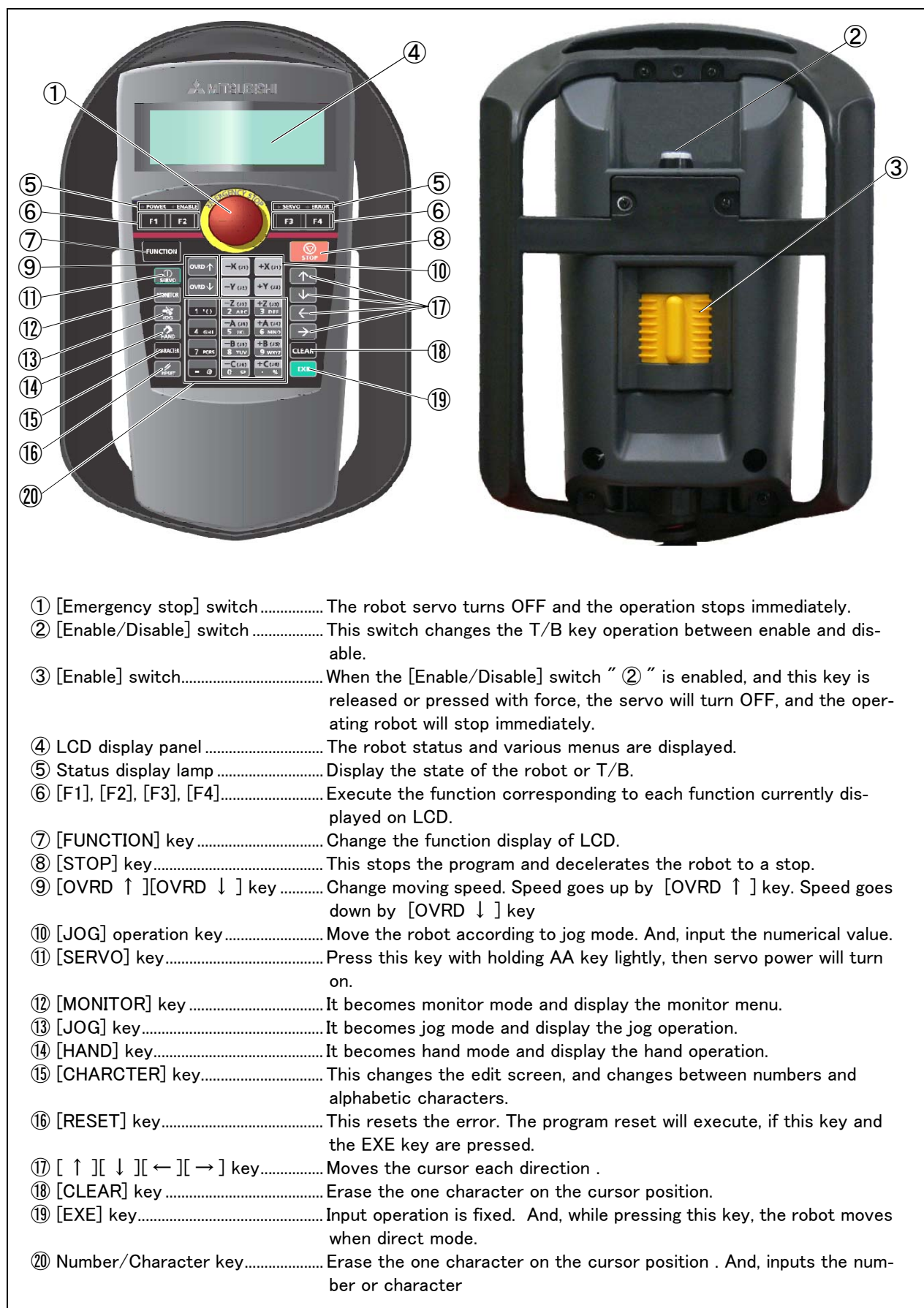
Fig.3-26 : Teaching pendant key layout and main functions
