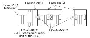
The FX2N-GM-5EC cable is used to connect the FX2N-10GM to an FX2N PLC. When along distance is required, one FX2N-GM-65EC cable can be used per system. To connect to an FX2NC PLC, the FX2NC-CNV-IF must be used. Eight blocks may be connected to an FX2N PLC and four blocks may be connected to an FX2NC PLC.
