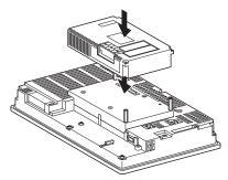
(7) Fasten the unit fixing brackets (3 places) with tightening torque of 0.36 to 0.48N•m.
