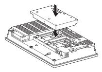
(4) Fasten the GT15-75IF900 by tightening its mounting screws (3 places) with tightening torque 0.36 to 0.48 N $\cdot$ m.
