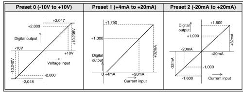
NOTE: Preset ranges are selected by an appropriate setting in the buffer memory of the analog block.
