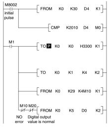
The ID code for the special function block at position "0" is read from BFM #30 of that block and stored at D4 in the main
