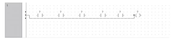
The pen can then strike through all contacts, from the bus bar, to the coil. In the Ladder Editor the suggestion is to invoke the *Auto Connect* feature when dropping elements onto the POU body or connecting parallel elements. It should however be disabled when connecting a row of contacts as shown in the following screen, or inserting a contact into an existing network.
