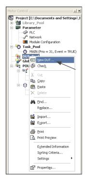
⑤ Create a new DUT by right clicking on the **DUT Pool** icon in the Program navigation window
