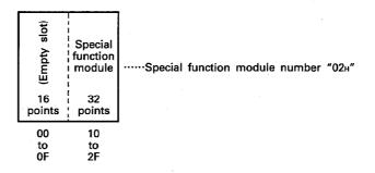
(c) Module occupying two slots and using the second slot as empty
