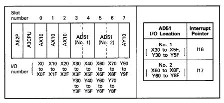
Fig. 7.7 System Configuration and Interrupt Pointers
