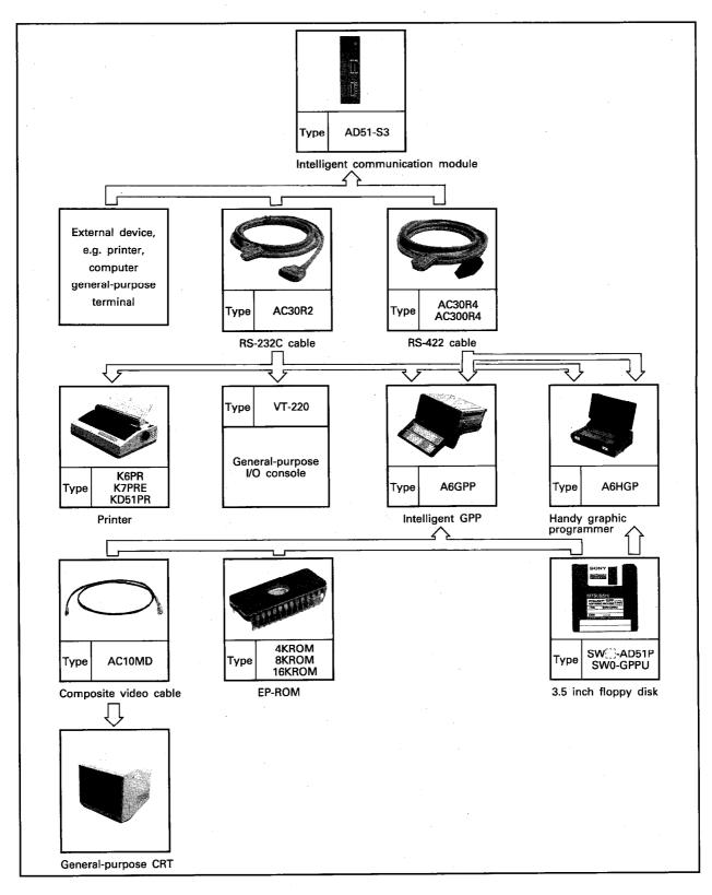
Fig. 2.3 Peripheral Device Configuration
