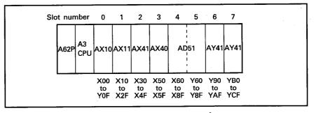
Fig. 7.2 Module Configuration
