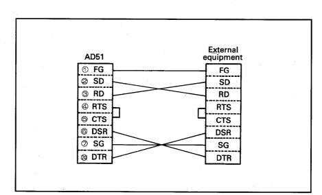
Fig. 5.1 RS-232C Connection Diagram
