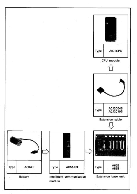
Fig. 2.2 Compact CPU Configuration
