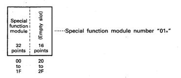
(d) Module occupying two slots as a special function module and an input module (A81CPU)
