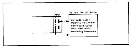
(5) Connection of AD51 and external device
