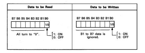
(b) When a system subroutine has been called with "word" specified, and bit devices are to be processed (i.e. in batches of 16 devices) then one word of AD51 memory is used per 16 bits.
