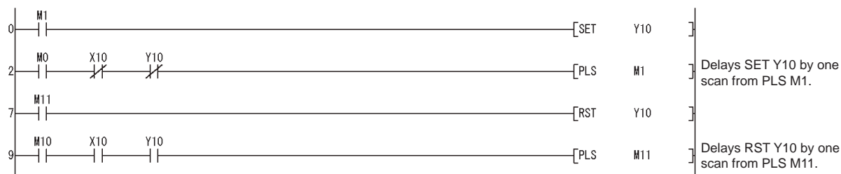
Diagram 7.17 Program Example when there is Response (Input) to Output
