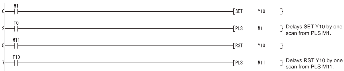
Diagram 7.20 Program Example when Outputting by timer contact
