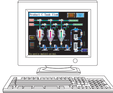
When the full screen mode function is used, the part of the frame is hidden and the full monitor screen can be displayed on the personal computer.
