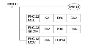
In Current Output mode, the user digital range of A  $\sim$  B is used to output a current of 4 - 20 mA. The range of A  $\sim$  B stored in D70 must be converted to a range of 0  $\sim$  2000 per the example program below.
