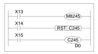
Counter C245 also has an external start contact, again automatically assigned. This is actually input X7. Once again this data can be found on the previous counter tables.
