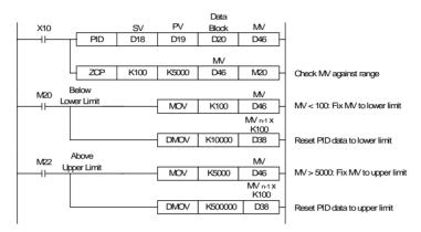
If data registers are used to hold the limit values, it is possible to use a MUL instruction instead of the DMOV. E.g. When D50 is upper limit use: MUL D50 K100 D38 because the result of MUL is already a double word DMUL is not needed.
