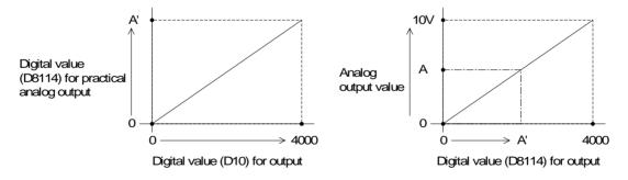
Because A is smaller than 10 Volts, the digital value of  $0\sim4000$  must be converted to a value of  $0\sim$ A' as shown in the graphs above. 4000/10V = A'/A or  $A' = [4000/10] \times A = 400 \times A$  D8114 =  $[A'] \times (D10 / 4000) = [400 \times A] \times [D10 / 4000) = (A \times D10) / 10$ .
