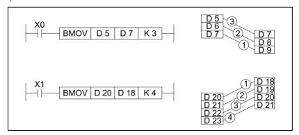
d) Using file registers as the destination devices [D]may be performed on all units.
