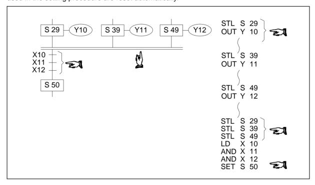
Because more than one state is being simultaneously joined with further states (some times described as a parallel merge), a set of horizontal parallel lines are used to aid a quick visual recognition.
