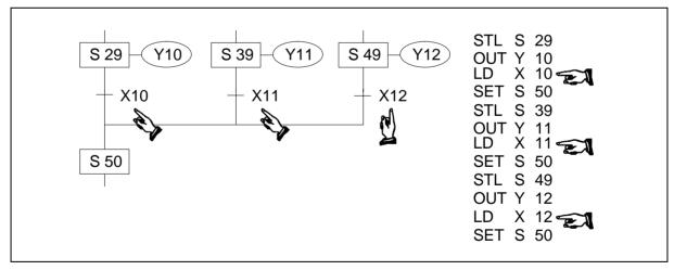
This type of STL program construction is called a "First State Merge" simply because the first state (in the example S29, S39 or S49) to complete its operation will cause the merging state (S50) to be activated. It should be noticed how each of the final STL states on the different program branches call the same "joining" STL state.
