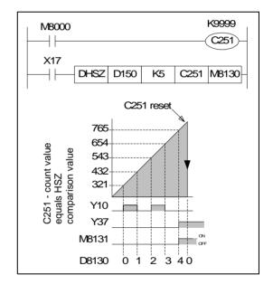
When the DHSZ instruction is initially activated it will not process a comparison until the following program scan as the CPU requires a slight time delay to initialize the comparison table.
