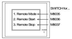
The HMI should be programmed with 'SWITCH' devices driving the three special M codes M8035,36 and 37. By activating the 'SWITCH' devices for M8035 and M8036 the PLC can be switched into a RUN state, while driving the 'SWITCH' device M8037 will put the PLC into a STOP state.
