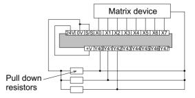
f) Because this instruction uses a series of multiplexed signals it requires a certain amount of 'hard wiring' to operate. The example wiring diagram to the right depicts the circuit used if the previous example instruction was programmed. As a general precaution to aid successful operation diodes should be places after each input device (see diagram opposite). These should have a rating of 0.1A, 50V.
