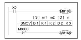
To select the BCD mode the SMOV instruction is coupled with special M coil M8168 which is driven ON. Please remember that this is a 'mode' setting operation and will be active, i.e. all SMOV instructions will operate in BCD format until the mode is reset, i.e. M8168 is forced OFF.
