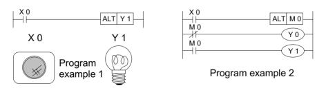
Pressing the momentary push button X1 once will switch the lamp ON. Pressing the push button for a second time will cause the lamp to turn OFF. And if the push button is again pressed for a third time, the lamp is turned ON again and so the toggled status continues. The second program shown identifies a possible motor interlock/control, possibly a start/stop situation.
