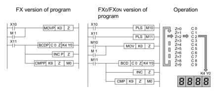
until it equals 9. When this happens the comparison instruction drives M1 ON which in turn resets the current value of Z to 0 (zero). Hence, a loop effect is created with Z varying between fixed values of 0 and 9 (10 values). The Z value is used to select the next counter to be displayed on the seven segment display.
