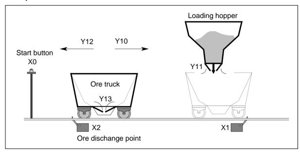
This simple example is an excerpt from a semi-automatic loading-unloading ore truck program. This example program has a built in, initialization routine which occurs only when the PLC is powered from OFF to ON. This is achieved by using the special auxiliary relay M8002.
