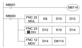
The desired analog output is from values A to B where 0 < A < B < 10 and the digital values range from  $0 \sim 4000$  in D20.
