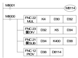
If using a digital range of C  $\sim$  D in the program to output an analog value of A  $\sim$  B, the digital value must be converted to the 0  $\sim$  4000 equivalent and the analog value must be converted to 0  $\sim$  10 Volt equivalent.
