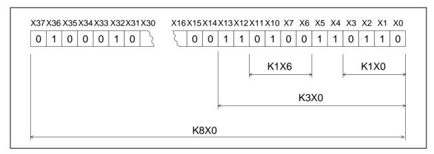
K1X0 : X0 to X3 ⇒ 4 bit devices with a head address of X0
