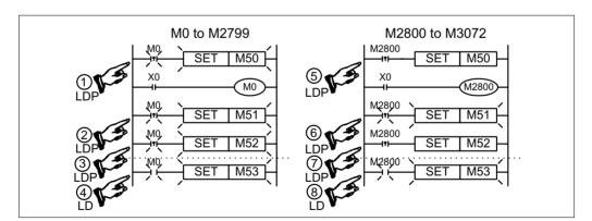
Turning ON X0 causes M0 to turn ON.
