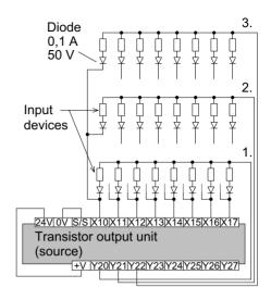
going OFF and Y22 coming ON. This then allows all of the inputs in the third bank to be read and stored in devices M50 to M57. The processing of this instruction example would take  $20 \times 3 = 60$ msec.
