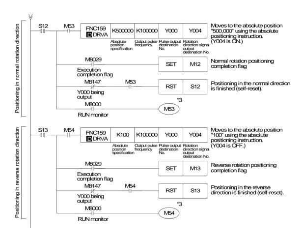
\*3 The instruction drive timing is delayed by one opeation cycle to prevent simultaneous driving of positioning instructions.
