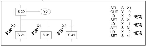
A programming construction to split the program flow between different branches is very useful but it would be more useful if it could be used with a method to rejoin a set of individual branches.
