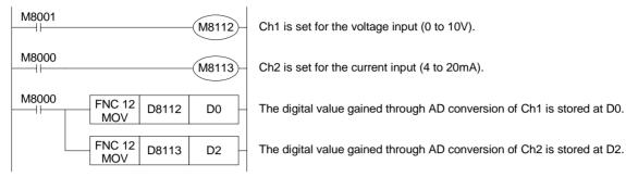
D0 ranges from 0 ~10000. To convert D0 to the 0 ~ 4000 value needed for D8114:  $D8114 = [D0 \times 4000] / 10000 \text{ or } [D \times 2] / 5$
