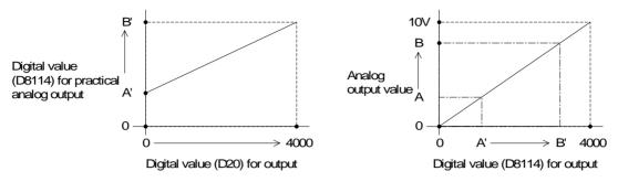
This example is equivalent to setting an offset and gain for the analog output.
