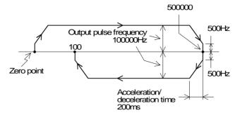
In this example the actual output frequency for the first step, acceleration, and the last step, deceleration, can be obtained using the following expression.
