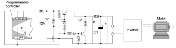
Circuit configuration for a PLC with sink outputs.
