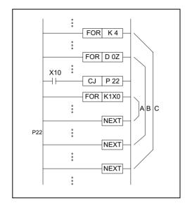
Number of loop C operations = 4 times Number of loop B operations = 24 times ( $C \times B$ ,  $4 \times 6$ ) Number of loop A operations = 168 times ( $C \times B \times A$ ,  $4 \times 6 \times 7$ )
