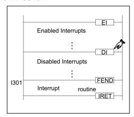
If an individual interrupt is to be disabled its associated special M coil must be driven ON. While this coil is ON the interrupt routine will not be activated. For details about the disabling M coils see the PLC device tables in chapter 8.
