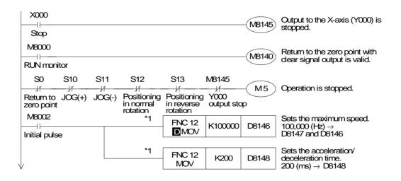
\*1 When the maximum speed or Acceleration/deceleration do not have to be changed from their initial values, programming is not required.
