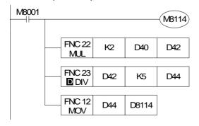
In the Current Output Mode, the 1DA converts values from  $0 \sim 2000$  to the analog output of  $4 \sim 20$  mA. If using a digital range of  $0 \sim 20000$  in the program, the range must be converted to  $0 \sim 2000$  as shown in the programming example below. Digital values for conversion to analog are stored in D8114.
