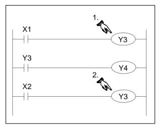
Double or dual coiling is not a recommended practice. Using multiple output coils of the same device can cause the program operation to become unreliable. The example program shown opposite identifies a double coil situation; there are two Y3 outputs. The following sequence of events will occur when inputs X1 = ON and X2 = OFF;
