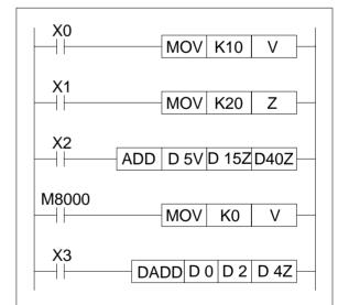
Both V and Z registers are initially set to K10 and K20 respectively.
