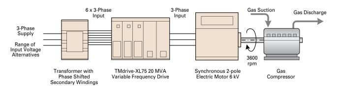
The TMdrive-XL75 variable frequency drive is designed to meet Oil & Gas industry needs for:
