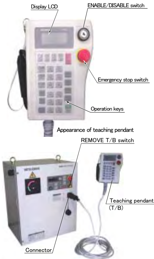
Fig.2-7 : Installing the T/B (control power OFF)
