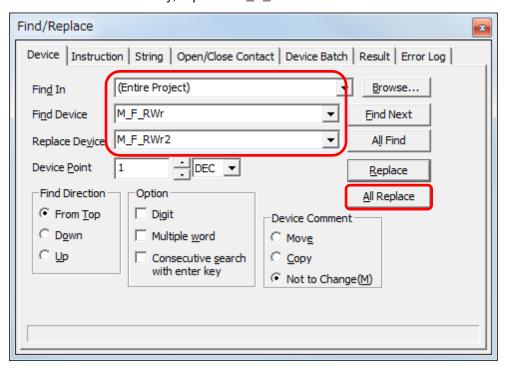
By performing the steps above, the CC-Link IE field master/local FB can be used for the second module.
