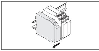
⇒ If there are several modules, slide the modules away from each other individually in the direction of the arrow until the side plug connection is separated.
