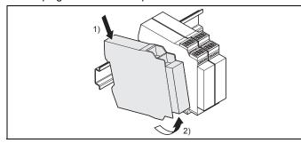
⇒ Press the module downwards at the rear 1) and remove it from the DIN rail in the direction of the arrow while keeping it pressed down 2).
