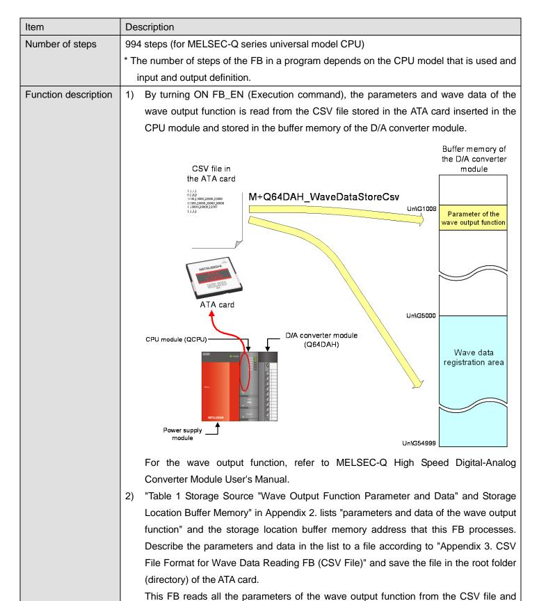
stores them in the buffer memory areas Un\G1008 or later. Then, this FB reads "Wave data" specified in "Number of wave data" of the line 100 in the CSV file from the line 101 in order for the number of specified points, and stores them into the start address (Un\G5000) or later of the wave data registration area of the buffer memory.
