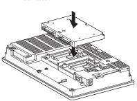
(4) Fasten the bus connection unit by tightening its mounting screws (4 places) with tightening torgue 0.36 to 0.48 N·m.
