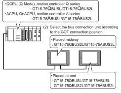
When using the bus connection, make the communication settings to perform communication between the GOT and PLC. Refer to the GOT1000 Series Connection Manual for details of
