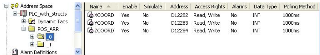
Array[0..1] of POSITION variables
