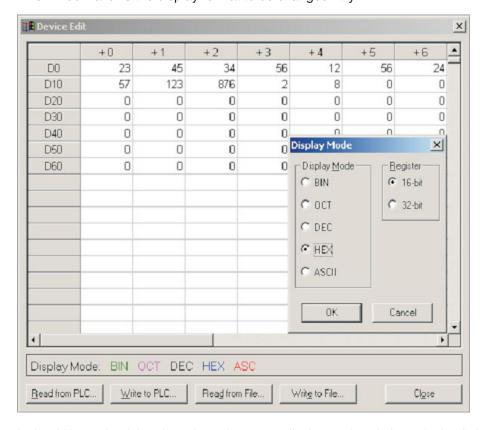
It should be noticed that the selected row now displays values in hexadecimal, the other values remain unchanged. In fact, individual cells can have different display formats, making this feature extremely flexible.
