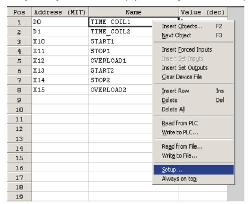
The *Setup* window allows the EDM to be user configurable; clicking the right mouse button, displays the configurator window. In this procedure Columns will be added to the EDM table for IEC Address and Hex Value Monitor.
