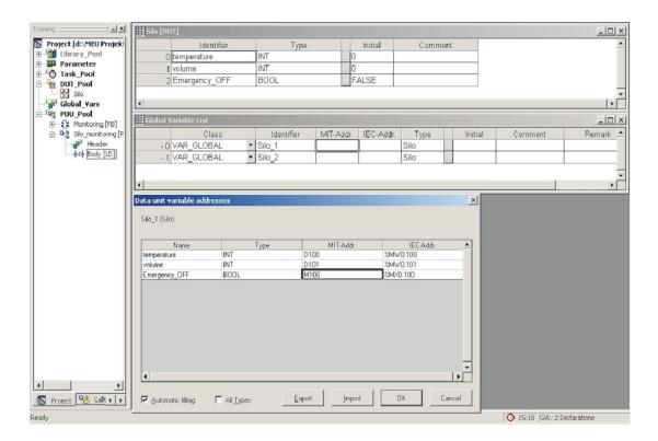
To view all definitions at once (if more than one definition is available), DUT entries in the GVL can be expanded by double-clicking the row number field.
