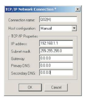
③ Then make the following settings for Controller 1 (i.e. the target PLC), according to the settings made in the PLC earlier.
