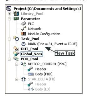
② Double click on the task and bind the POU "MOTOR\_CONTROL" to the task "MAIN":
