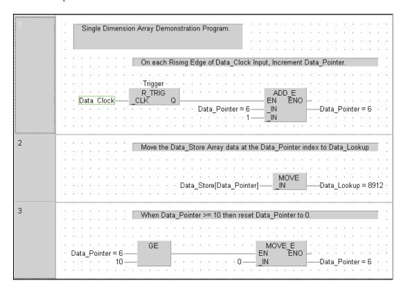
The program is designed to reset the pointer to zero on the 10<sup>th</sup> element and thus will repeat scan the table with an upward increment (Index 0-9). Working with Libraries
