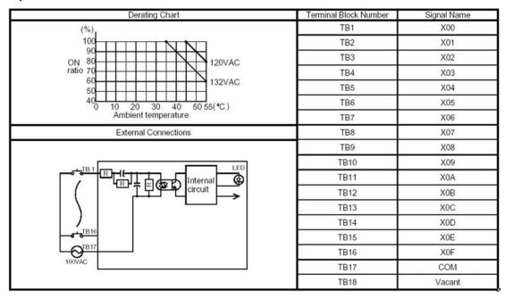
With AC Input type modules, it is recommended that the same supply voltage to the PLC is used as for the inputs i.e. (100 - 120VAC). This minimises the possibility of an incorrect voltage being connected to the Inputs.
