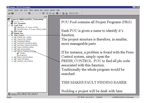
Above an example of the GX-Developer display is shown illustrating an example POU Pool.
