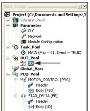
The new DUT will now be displayed under the **DUT Pool** in the project.
