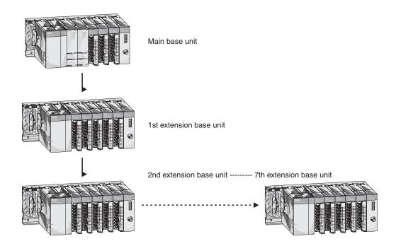
The base unit and extension units are simply connected to one another by extension cables. These connecting cables also supply the extension units with the operating voltage of 5 V DC.
