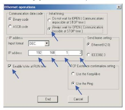
After the settings here are made, click *End* to return to the main network parameter setting window. Note that the *Operational settings* button has now changed to blue, indicating that changes have been made.
