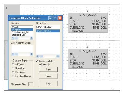
② Assign 'instance names' to both instances of the Function Block, STAR\_DELTA by typing MCC1 and MCC2 into the Instance names above each Instance of the FB. At the system prompt, click **Define Local**.
