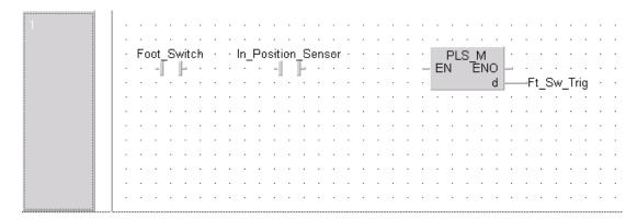
Finally, the ladder network must be finalised by connecting up the elements as follows.
