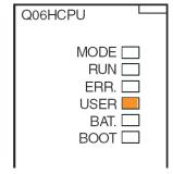
ON: After the detection of an error during self-diagnostics.
