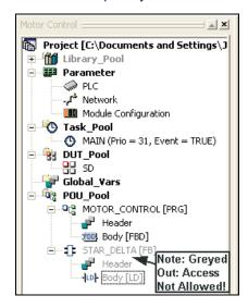
Access attributes for <u>any</u> individual object or complete folder in the 'Project Navigation Window' above can be individually set, allowing higher degrees of flexibility in the program security settings.
