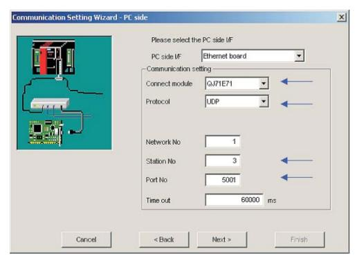
⑤ Configure the Communication settings of the PLC side required for the example system described earlier.
