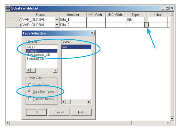
The variables are stored in the Global Variable List. The structure of both variable, Silo\_1 and Silo\_2, is identical, so to reference the individual variable of each DUT you only need to prefix their names with the name of the respective global variable.
