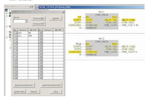
③ To toggle the status of X10 or X11, double click the left mouse button over the *ON/OFF* status cell.
