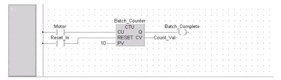
When entering the PV and CV values, use the variable water buttons respectively.
