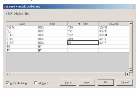
4 Finally, enter the two remaining Integer Variables TB and TV using MELSEC addresses D0 and D1 using the "Auto Fill" feature:
