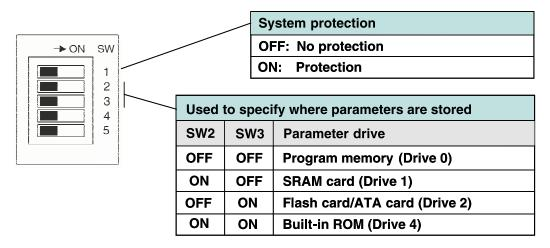
Parameters can not be stored in the built-in RAM (Drive 3).
