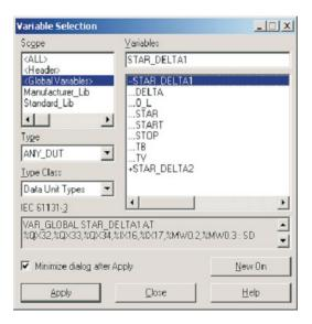
4 Pick and assign the variables to the two STAR\_DELTA Function Blocks on the MOTOR\_CONTROL Program POU as shown:
