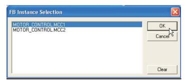
② Select the instance of the Function Block MOTOR\_CONTROL.MCC1 and observe the monitored page:
