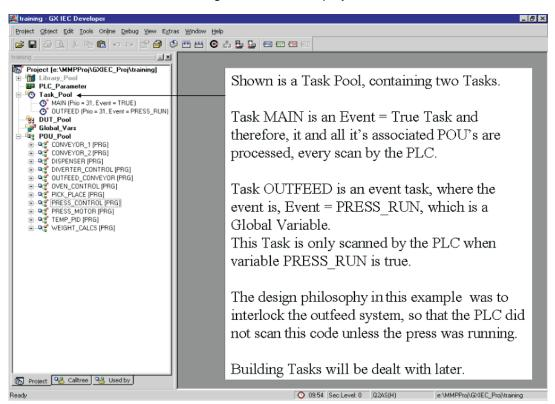
The **Task Manage**r allows the user to efficiently manage the PLC scan, ensuring that only the routines that require scanning are executed. It also provides an easy method of allocating specific routines to events and timed or priority interrupts.
