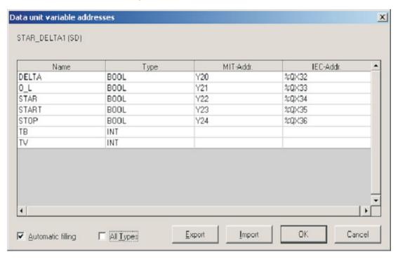
The system will try to sequentially 'Auto Fill' the variables of type BOOL. Although in many situations this is recommended, in this case it is only partially successful.
