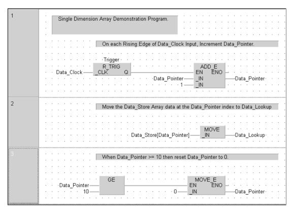
Note: Define the 'R\_Trig' Function block with instance name "Trigger".
