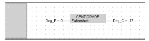
② Using the on screen variable forcing feature, input numbers into the 'Deg\_F' variable as follows:
