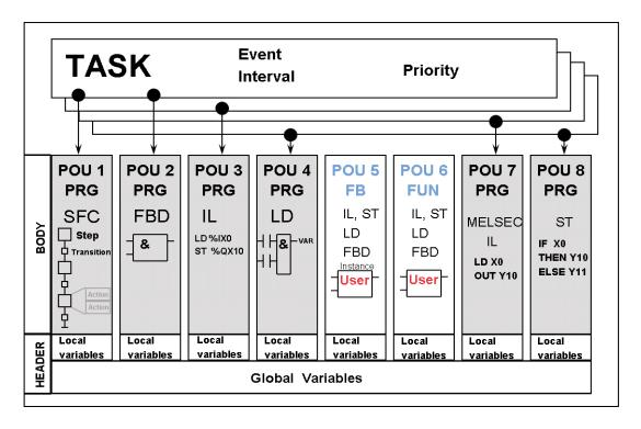
Overall Project Configuration illustrating POU integration using SFC, FBD, IL, LD and MELSEC IL and ST format programs.
