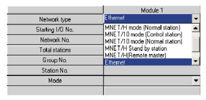
(5) The dialogue box now shows the specific setting options for the module. The buttons in the bottom half of the table that are in red are for setting the mandatory parts of the module, those in magenta are optional, and are set as required.
