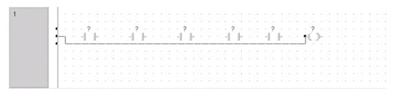
The pen can then strike through all contacts, from the bus bar, to the coil. In the Ladder Editor the suggestion is to invoke the *Auto Connect* feature when dropping elements onto the POU body or connecting parallel elements. It should however be disabled when connecting a row of contacts as shown in the following screen, or inserting a contact into an existing network.
