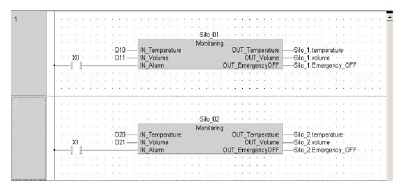
The GVL has been extended to define addresses for all elements of data unit types. Not defined addresses are handled by the system.
