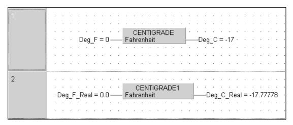
Modify the value of the input variable "Deg\_F\_Real" and observe the output result on the display. Note the 7 Digit floating point accuracy.
