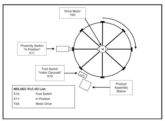
There are a number of issues that must be addressed when designing a PLC program for the above application. Using a standard Start / Stop circuit is not possible without modification due to the following difficulties:
