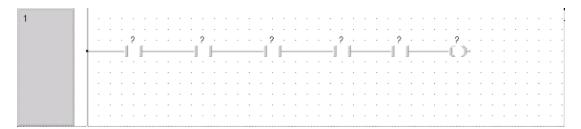
When using multi-legged or 'pinned' functions such as MUL, the number of input parameter legs, can be incremented/decremented by using the special toolbar, icons shown. This can also be achieved by placing the cursor at the bottom edge of the function, holding down the left hand mouse button and then dragging away as shown below:
