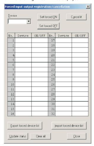
② Enter X10 and X11 into the **Device** dialogue box and click on the **Set Forced ON** button for both variables:
