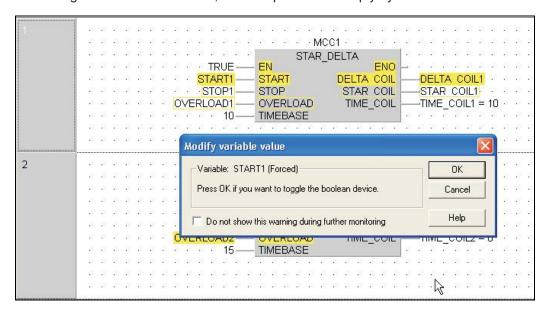
For Integer/Real variables, use the same procedure, i.e. double click on the variable name, whilst in monitor mode. The new value can be entered either as decimal or as a hexadecimal value.
