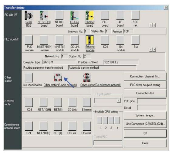
This will complete the setting, making the dialogue look as shown below. Click Connection test to confirm the settings are correct. Then click OK when finished.
