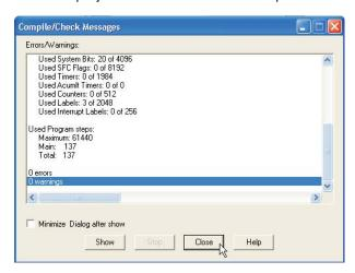
Download and monitor the project. Before the Function Blocks can operate, it is necessary to write values into the TIMEBASE inputs: STAR\_DELTA1.TB and STAR\_DELTA2.TB. This is carried out by using the online variable modification technique described in an earlier section.
