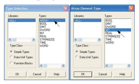
Note that when the array entry first appears, it will be dimensioned to the default value of ARRAY [0..3] OF INT. It is necessary to re dimension it to [0..9] of INT for this example, as shown below:
