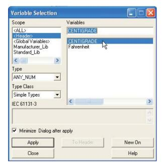
CENTIGRADE is automatically placed in the header variable list as it is the name of the function, it must therefore also be specified as the output argument.
