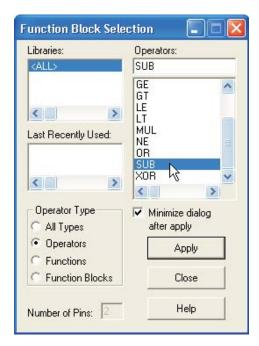
② Using Apply or double clicking on the selection object, place it on the screen:
