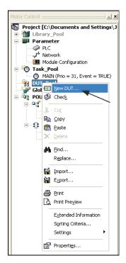
⑤ Create a new DUT by right clicking on the *DUT Pool* icon in the Program navigation window
