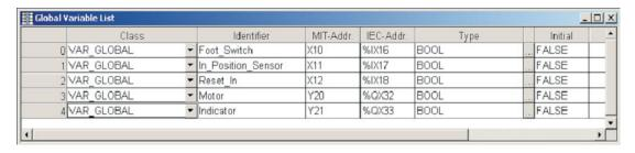
The header (LVL) for the above program "Batch\_Count" should now appear as shown:
