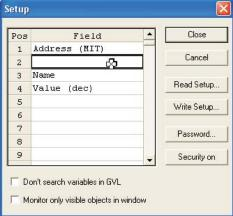
③ Double click on the empty field or press F2 and select *Address* (*IEC*) from the list as shown.
