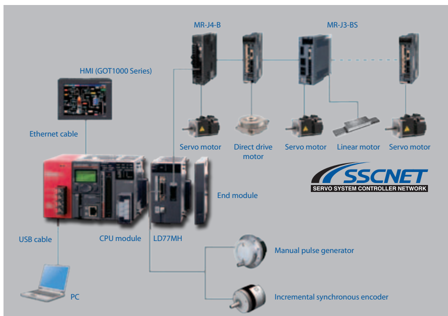
Structure of a system configuration comprising servo amplifiers and servo motors together with an L Series PLC-CPU.
