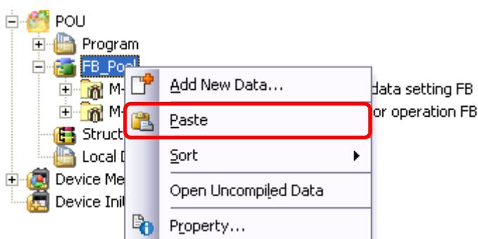
(3) After selecting the paste command, a window appears to enter an FB name. Enter an FB name after paste.
