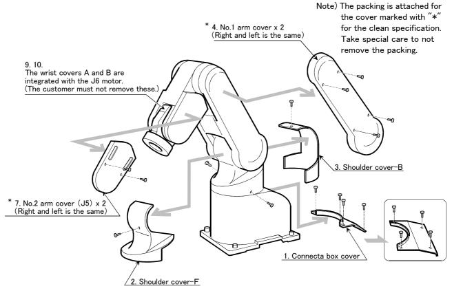
Fig.5-4: Installing/removing the cover (5-axis type)
