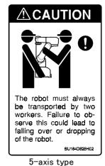
Fig.2-2: Transportation of robot arm
