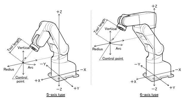
\* The current position is set as the arc centering on the Z axis, and the axis moves along that arc, expands and contracts in the radius direction, and moves vertically. At this time, for the 6-axis type, the flange surface posture is maintained. Also, while maintaining the flange surface position, the flange surface posture changes.
