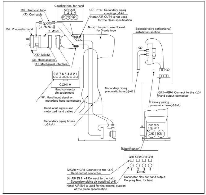
Fig.3-2: Pneumatic hand set installation procedures
