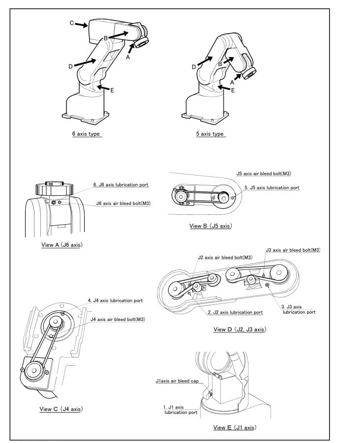
Fig.5-11: Lubrication positions
