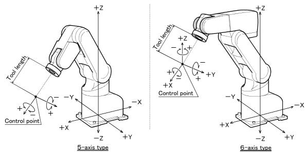
\* While maintaining the flange surface posture, the axis moves straight along the base coordinate system.
