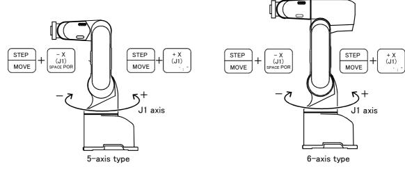
When the [MOVE] + [+X (J1)] keys are pressed, the J1 axis will rotate in the plus direction.
