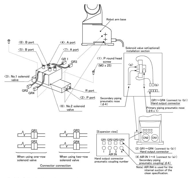
Fig.3-1: Solenoid valve installation procedures
