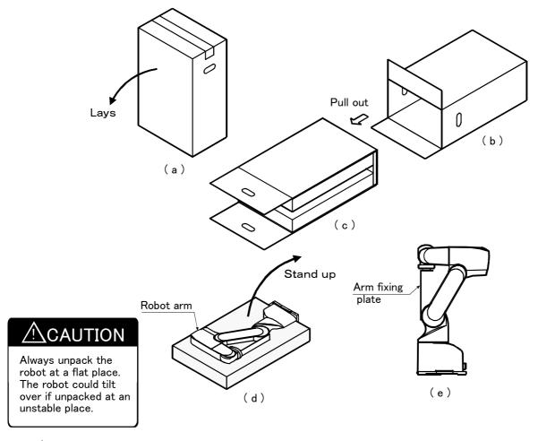
Note) The cushioning material will be required if the robot is transported again, so save it in a safe place.
