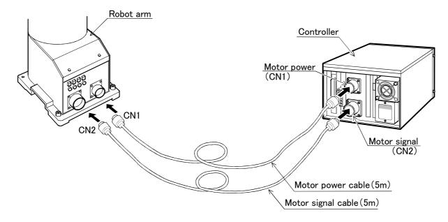
Fig.2-6: Connecting the machine cables
