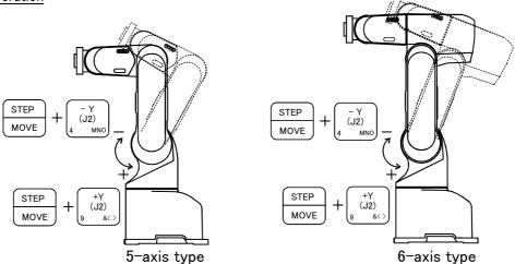
• When the [MOVE] + [+Y (J2)] keys are pressed, the J2 axis will rotate in the plus direction. When the [MOVE] + [-Y (J2)] keys are pressed, Rotate in the minus direction.
