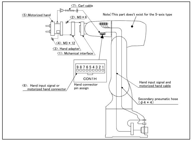
Fig.3-4: Motorized hand set installation procedures
