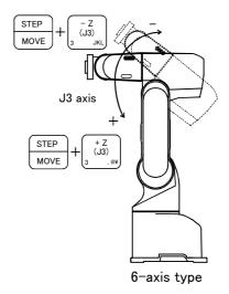
• When the [MOVE] + [+Z (J3)] keys are pressed, the J3 axis will rotate in the plus direction. When the [MOVE] + [-Z (J3)] keys are pressed, Rotate in the minus direction.
