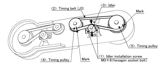
Fig.5-7: Inspection, maintenance and replacement of J3-axis timing belt
