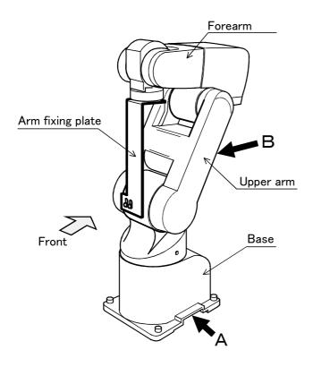
Note) The figure shows the 6-axis type, but this also applies for the 5-axis type.
