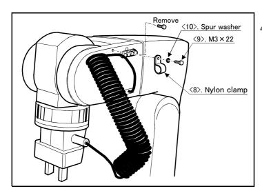
Fig.3-5: Fix the motorized hand cable
