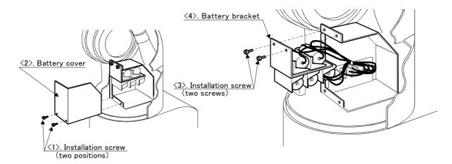
Fig.5-12: Replacing the battery
