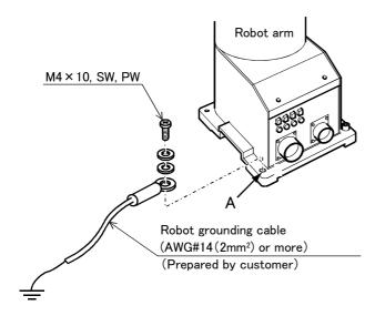
Fig.2-5: Connecting the grounding cable
