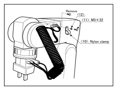
Fig.3-3: Fix the air hand cable
