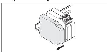
Remove the plug-in package terminals with wiring and the end clips.
