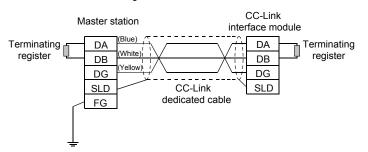
Use a bar terminal to connect the cable to the CC-Link interface module. For applicable bar terminals, see Chapter 8 Cable specifications. Two poles of each terminal are internally connected. (See below.)
