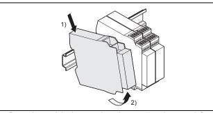
Press the module downwards at the rear 1) and remove it from the DIN rail in the direction of the arrow while keeping it pressed down 2).
