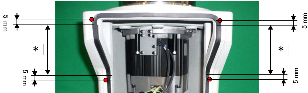
Fig.5-8 : Sticking the packing doubly (RV-12SD series)
