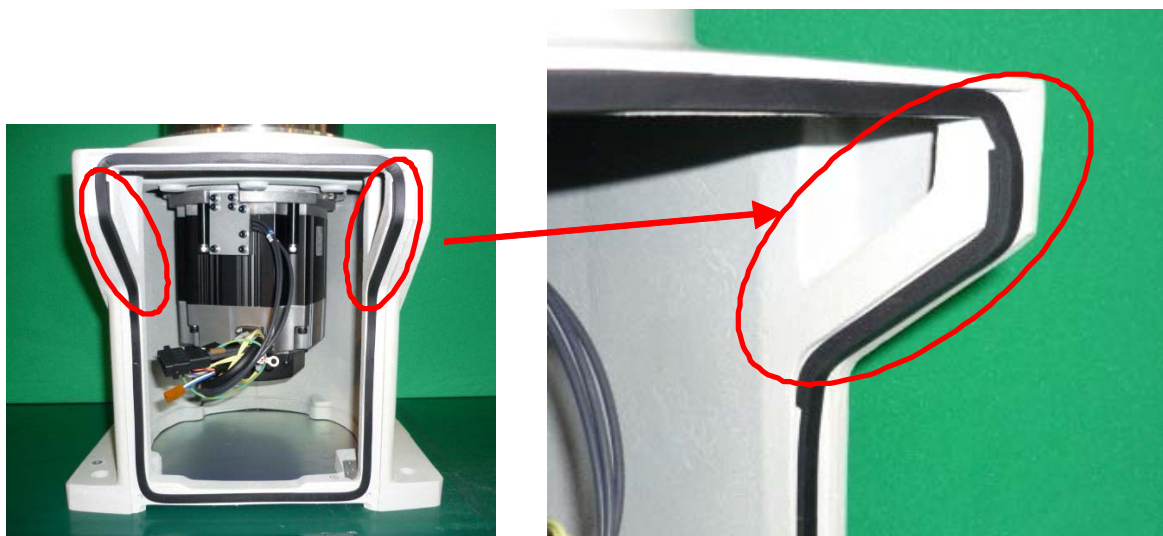
Fig.5-9 : Position of sticking doubly (RV-12SD series)
