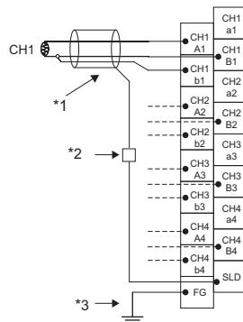
\*1 Use the conducting cable with shield and make the wiring length as short as possible.
