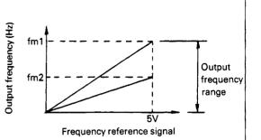
Note: The set maximum frequency changes automatically when setting of "gain for frequency reference voltage signal" (see p. 15-3) is changed. Since this function has the priority level same as that of 3rd function (C-3), priority is given to the latest set function, when this function is set together with a 3rd function.
