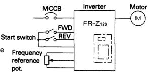
Fig. 6-1 Operation with external signals
