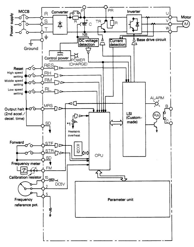
\*1:Heatsink overheat protection is not provided for FR-Z120-0.4K to 1.5K. Fig.9-1
