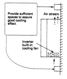
Fig. 4-1 Clearance around inverter
