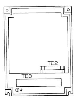
Control Circuit terminal block TE2 (M3.5 screw) 10 2 5 В С FM SD STFISTRI RL RM RH MRS RES SD Main circuit terminal block TE3 (M4 screw) R P PR S W Т U V  $\bigoplus \frac{\perp}{-}$  (M4 screw) Ground terminal
