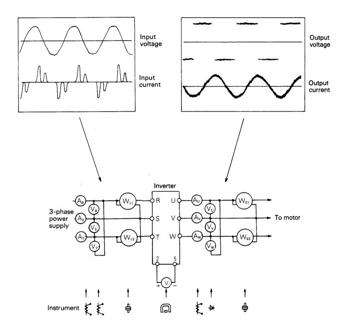
Fig. 7-2 Measuring points and instrumests
