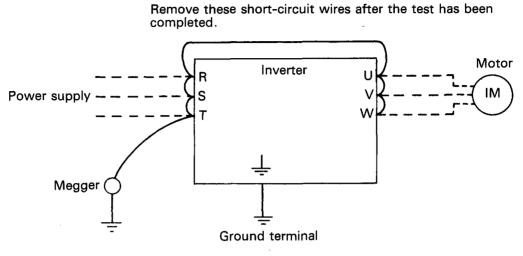
Fig. 7-1 Insulation resistance test with megger
