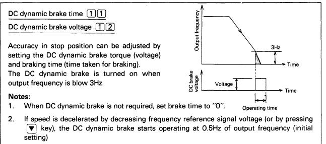
3. Initial setting of DC dynamic brake voltage ..... 8%
