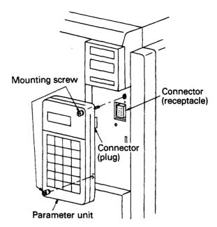
Fig. 2-7 Removal and installation of parameter
