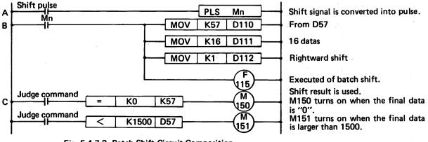
Fig. 5.4.7.3 Batch Shift Circuit Composition
