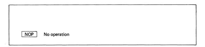
NOP is a no operation instruction and has no influence on the results of preceding arithmetic operation. An effective use of this instruction is to write NOP per desired step when preparing a program and to delete it when the program is completeld.
