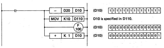
Fig. 5.4.14.2 Data Inversion Circuit
