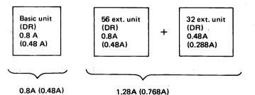
When capacity is calculated on the assumption that each unit has simultaneous 60% "ON" ratio, values in parentheses are obtained. In this case, power supply unit is added to the E56 extension unit in order to supply power also to the E32 extension unit.
