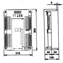
Fig. 8.2.1 External Dimensions of Basic Unit
