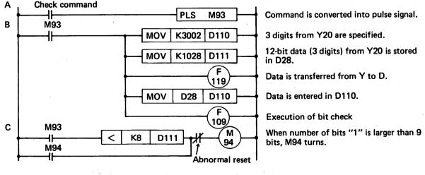
Fig. 5.4.13.3 Checking of Number of Bits "1" of Output Y
