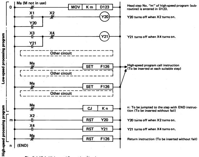
Fig. 5.4.15.1 High-speed Processing Circuit
