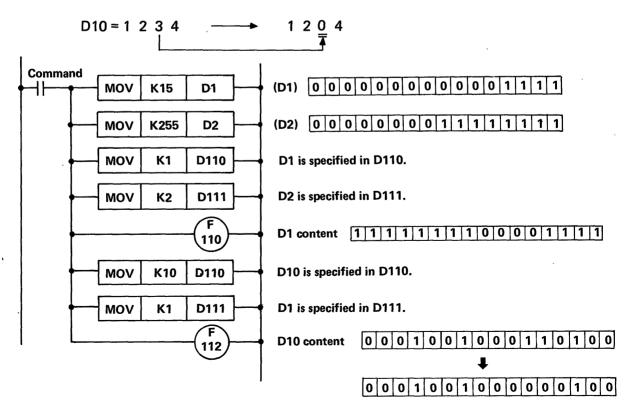
Fig. 5.4.4.2 AND Operation Circuit
