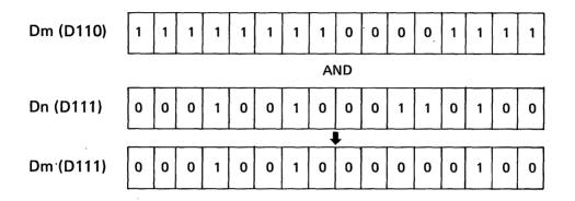
Fig. 5.4.4.1 16-bit data AND operation
