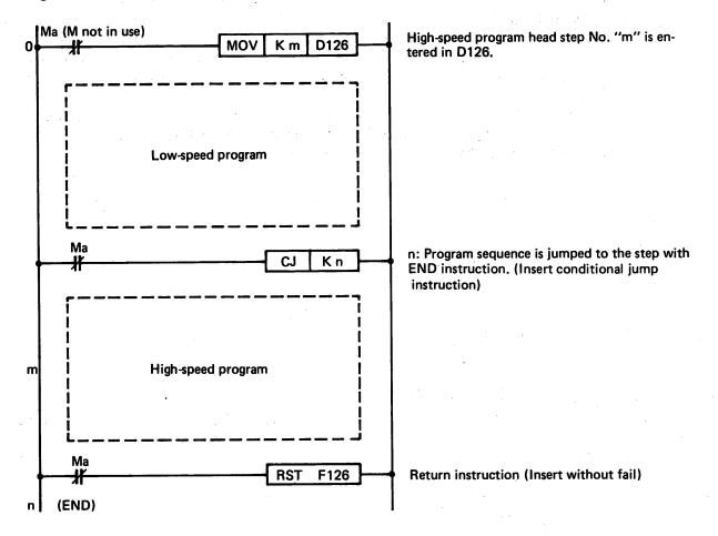
Fig. 5.4.15.3 Circuit for Programming with 10mS Timers
