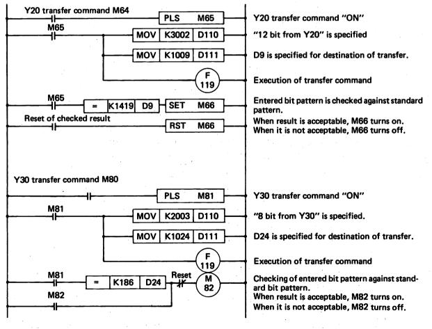
Fig. 5.4.11.2 Y → D Data Transfer Circuit
