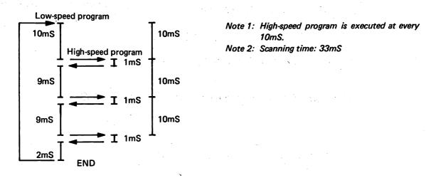
Fig. 5.4.15.4 Program Execution Flow Chart and Execution Time (When used with 10mS timer)
