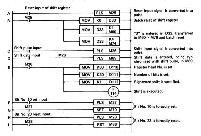
Fig. 5.4.6.7 Rightward Shift Register Circuit
