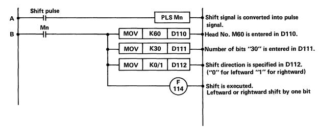
Fig. 5.4.6.1 Shift Register Circuit Composition
