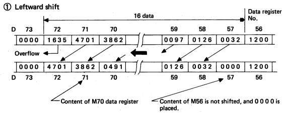
Fig. 5.4.7.1 Batch Shift (Leftward shift)
