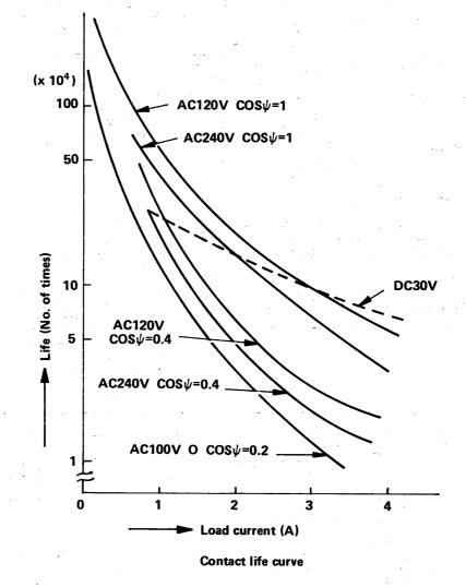
Note: When DC 100V load is opened and closed at the contact, set load current at 0.1 A or lower. When frequency is too high even at 0.1 A load, be sure to connect C-R surge killer or flywheel diode in parallel with the load.
