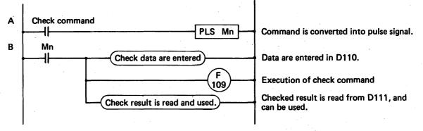
Fig. 5.4.13.1 16-bit Check Circuit Composition
