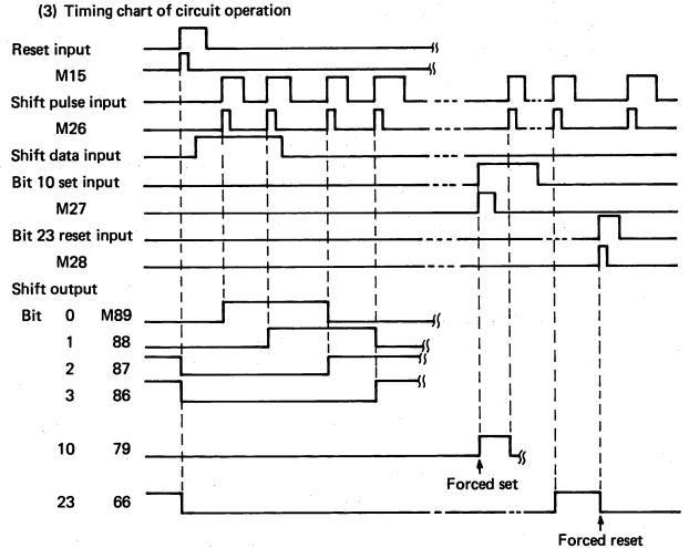
Fig. 5.4.6.8 Rightward Shift Register Timing Chart
