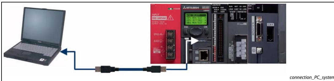
Fig. 2-16: Connection of PC and CPU module via USB
