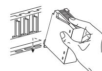
② Push the module in the direction of arrow to load it into the base unit.
