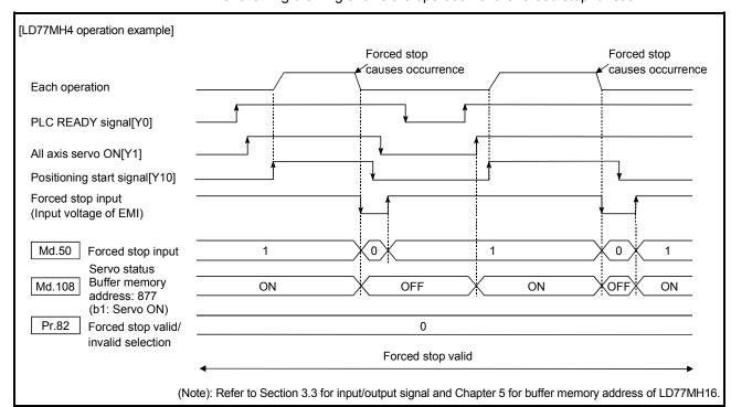
The following drawing shows the operation of the forced stop function.
