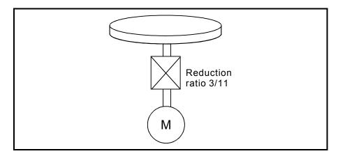
First, find how many degrees the load (machine) will travel ( $\Delta S$ ) when the motor turns one revolution (AP).
