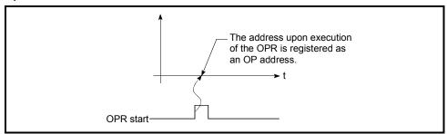
Fig. 8.9 Data set method OPR
