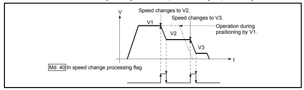
Fig. 13.22 Speed change operation
