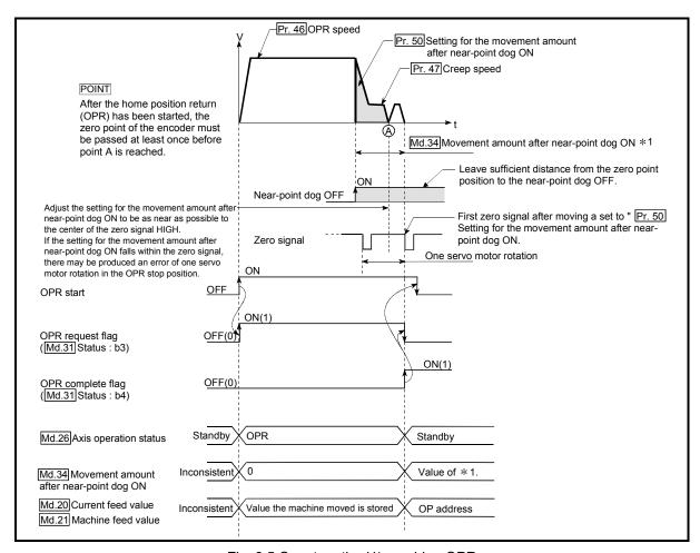
Fig. 8.5 Count method1) machine OPR
