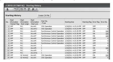
For the starting history check method, refer to the "Simple Motion Module Setting Tool Help" of GX Works2.
