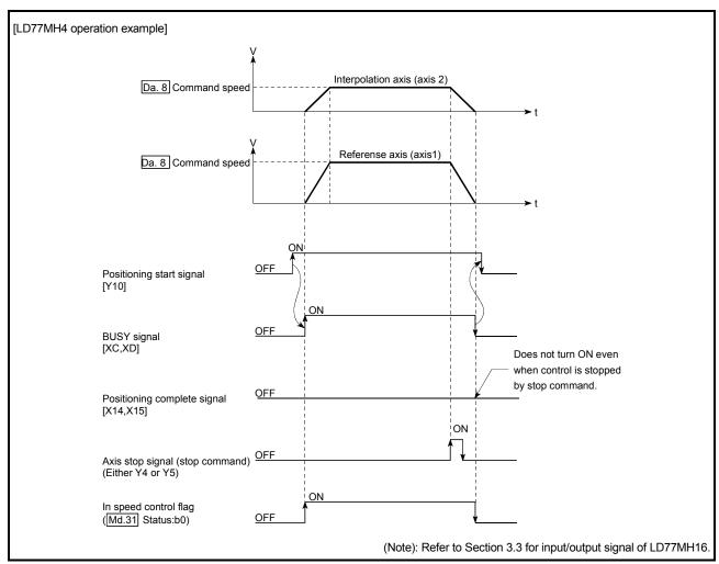
Fig. 9.10 2-axis speed control operation timing
