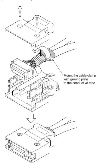
(6) To make this product conform to the EMC directive instruction and Low Voltage Directives, be sure to used of a AD75CK type cable clamp (manufactured by Mitsubishi Electric) for grounding connected to the control box and the shielded cable.
