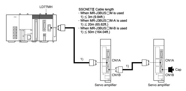
(Note): It cannot communicate with that the connection of CN1A and CN1B is mistaken.
