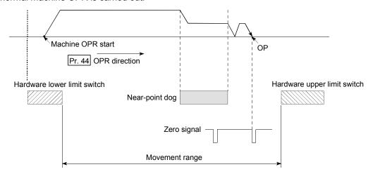
2) When the direction from the workpiece to the OP is the opposite direction from the " Pr.44 OPR direction", the operation carries out a deceleration stop when the near-point dog turns OFF, and then carries out a machine OPR in the direction set in " Pr.44 OPR direction".
