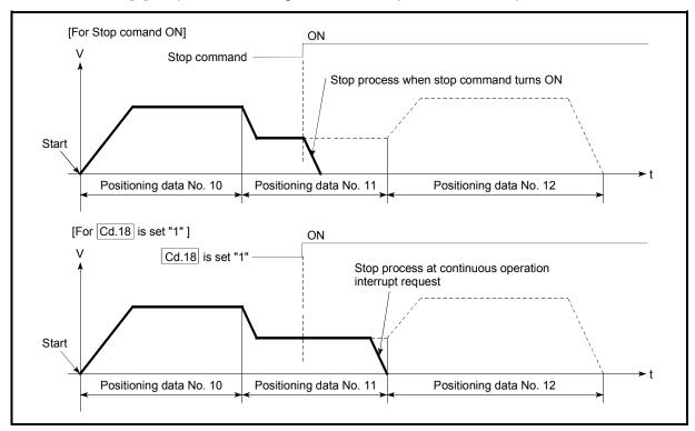
Fig. 6.12 Operation during continuous operation interruption
