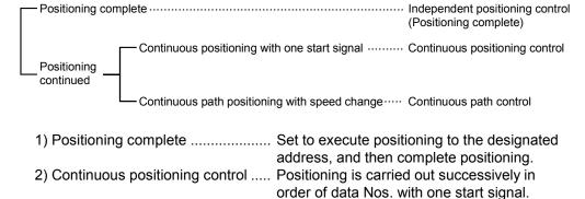
indicated by a positioning data. 3) Continuous path control...... Positioning is carried out successively in order of data Nos. with one start signal. The operation does not stop at each positioning data.
