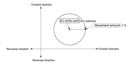
In circular interpolation control with center point designation, an angular velocity is calculated on the assumption that operation is carried out at a command speed on the arc using the radius calculated from the start point address and center point address, and the radius is compensated in proportion to the angular velocity deviated from that at the start point.
