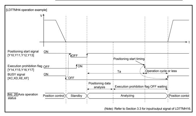
Fig. 13.48 Operations of pre-reading start function
