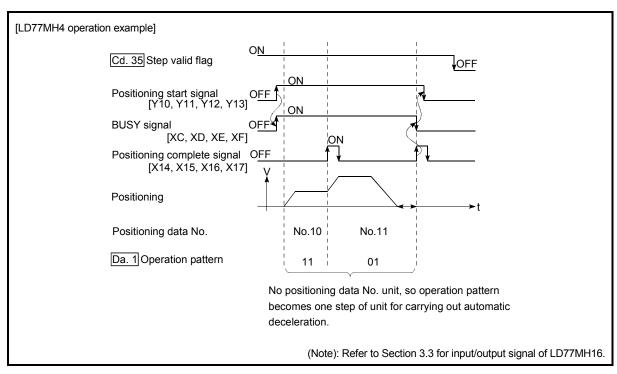
Fig. 13.37 Operation during step execution by deceleration unit step
