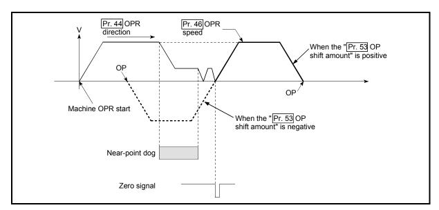
Fig. 13.6 OP shift operation at the OPR speed
