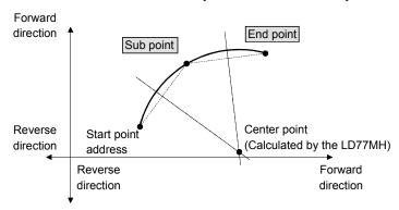
(b) Circular interpolation with the specified center point
