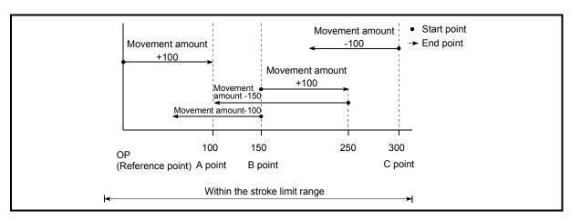
Fig. 9.7 Incremental system positioning
