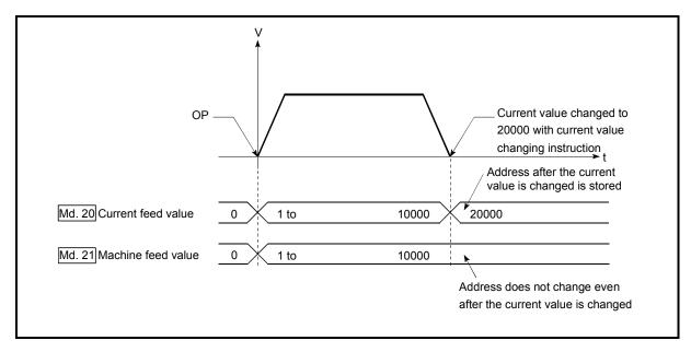
Fig. 9.8 Current feed value and machine feed value
