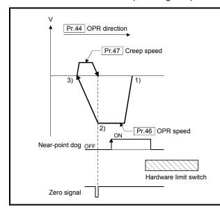
[Operation when a machine OPR is started from the near-point dog ON position]
