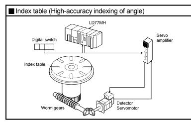
The index table is positioned at a high accuracy using the 1-axis servo.
