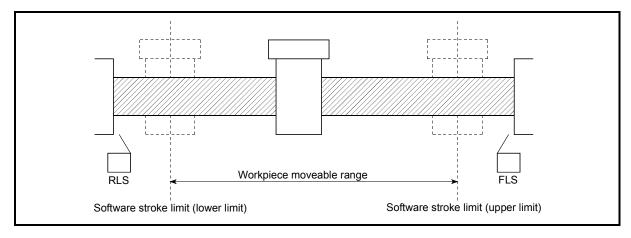
Fig. 13.13 Workpiece moveable range
