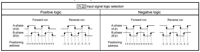
(b) A-phase/B-phase multiplied by 1 The positioning address increases or decreases at twice rising or twice falling edges of A-phase/B-phase.
