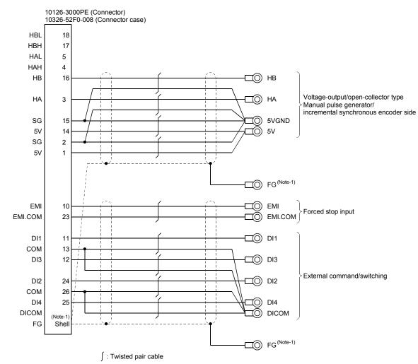
(Note-1): Ground FG terminal on the used equipment side. Also, connect it to the shell of connector side.
