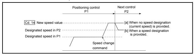
Fig. 13.23 Speed change during continuous path control
