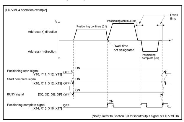
Fig. 9.2 Operation during continuous positioning control
