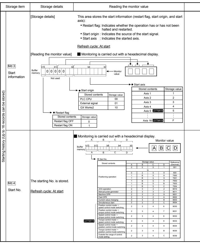
Note: If a start signal is issued against an operating axis, a record relating to this event may be output before a record relating to an earlier start signal is output.
