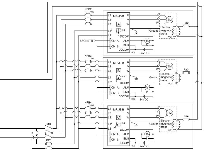
(Note-1): When the control power supply of servo amplifier is shut off, it is not possible to communicate with the servo amplifier after that. Example) When the control power supply L11/L21 of servo amplifier in above B figure is shut off, it is also not possible to communicate with the servo amplifier C.
