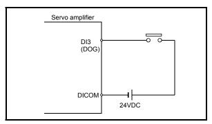
Fig. 8.1 Wiring when using the near-point dog
