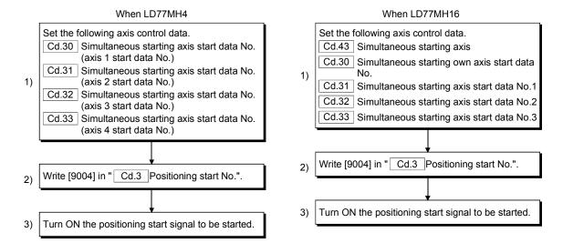
[4] Multiple axes simultaneous start control function setting method
