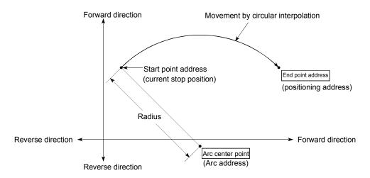
Positioning of a complete round with a radius from the start point address to the arc center point can be carried out by setting the end point address (positioning address) to the same address as the start point address.
