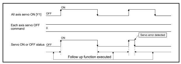
Fig. 13.54 Operation timings of follow up function
