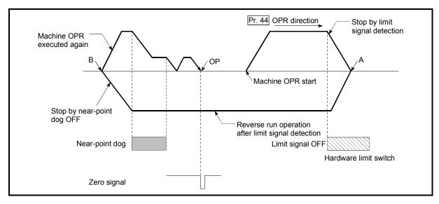
Fig. 13.3 Setting the dwell time during an OPR retry
