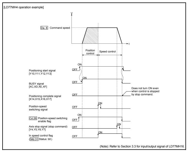
Fig. 9.18 Position-speed switching control operation timing
