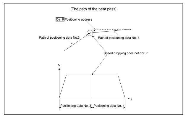
Fig. 13.9 The path of the continuous path control
