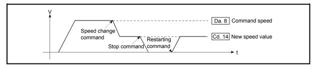
Fig. 13.24 Restarting speed after speed change made during position control
