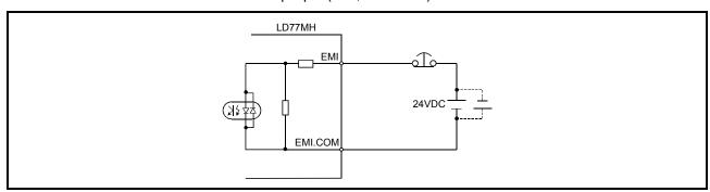
Fig. 13.21 Wiring when using the forced stop
