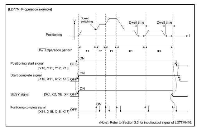
Fig. 9.4 Operation for the standard speed switching mode
