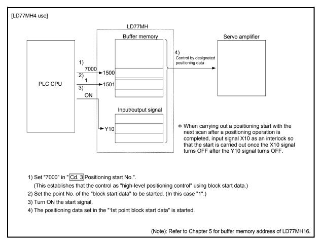
Fig. 10.2 High-level positioning control start procedure
