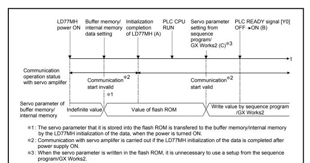
Fig. 7.1 Operation timing in the servo parameter transfer of the buffer memory
