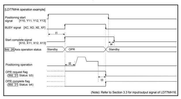
Fig. 6.9 Machine OPR operation timing and process time
