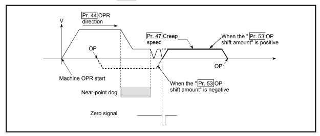
Fig. 13.7 OP shift operation at the creep speed
