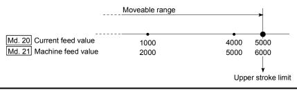
Fig. 13.14 Software stroke limits of the current feed value and machine feed value
