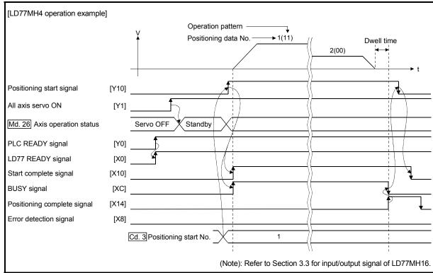
Fig. 6.6 Time chart for starting "major positioning control"
