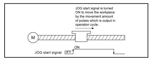
Fig. 11.2 Inching operation
