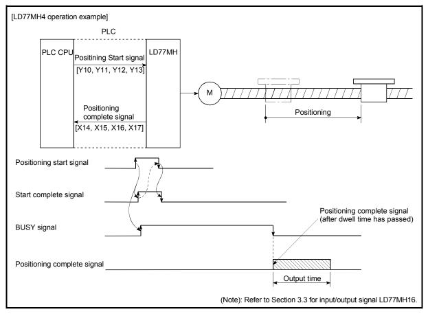
Positioning complete signal output time
