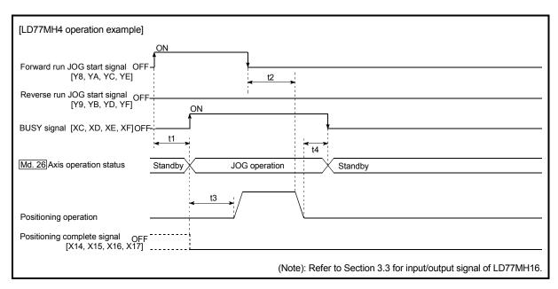
Fig. 11.5 JOG operation timing and processing times
