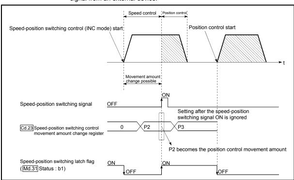
Fig. 9.15 Position control movement amount change timing
