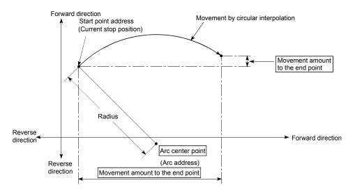
Positioning of a complete round with a radius of the distance from the start point address to the arc center point can be carried out by setting the movement amount to "0".
