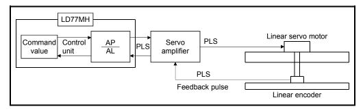
Calculate the number of pulses (AP) and movement amount (AL) for the linear encoder in the following conditions.
