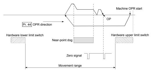
\* In the above example 1) and 2), "0: Positive direction" is set in " Pr.44 OPR direction"
