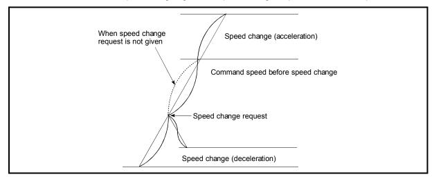
Fig. 13.47 Speed change during S-curve acceleration/deceleration processing
