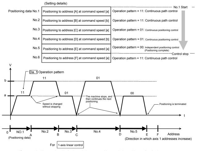
(One motor is driven, and positioning is carried out to an addresses designated in one direction.)
