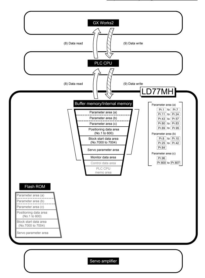
(8) Reading data from buffer memory/internal memory to GX Works2 ( )
