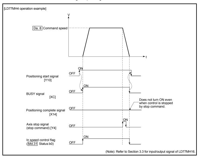
Fig.9.9 1-axis speed control operation timing
