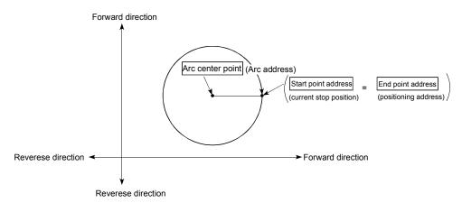
In circular interpolation control with center point designation, an angular velocity is calculated on the assumption that operation is carried out at a command speed on the arc using the radius calculated from the start point address and center point address, and the radius is compensated in proportion to the angular velocity deviated from that at the start point.
