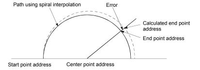
In circular interpolation control with center point designation, an angular velocity is calculated on the assumption that operation is carried out at a command speed on the arc using the radius calculated from the start point address and center point address, and the radius is compensated in proportion to the angular velocity deviated from that at the start point.
