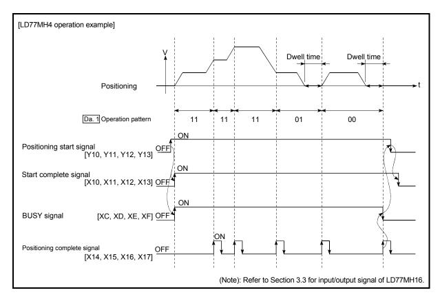
Fig. 9.5 Operation for the front-loading speed switching mode
