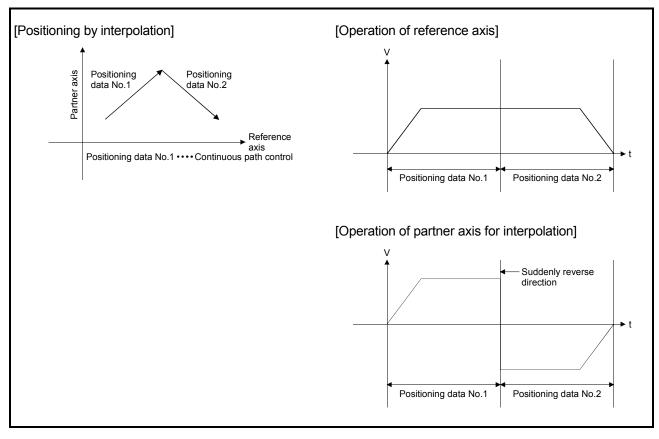
Fig. 13.10 Path and output speed of various axes when movement direction varies during continuous path control
