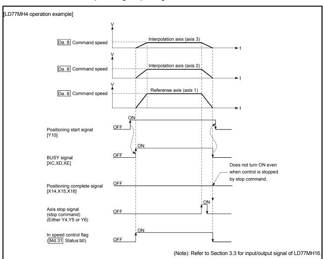
Fig. 9.11 3-axis speed control operation timing
