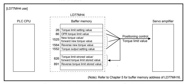
Fig. 13.12 Limiting the torque to the servo amplifier (Axis 1)
