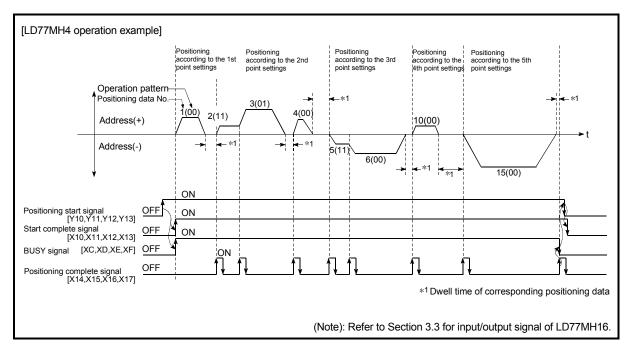
Fig. 10.1 Block start control example
