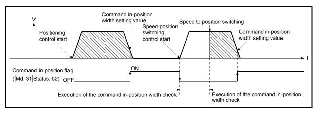
Fig. 13.44 Command in-position width check
