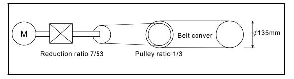
As the travel value of the conveyor is used to exercise control, set "mm" as the control unit.
