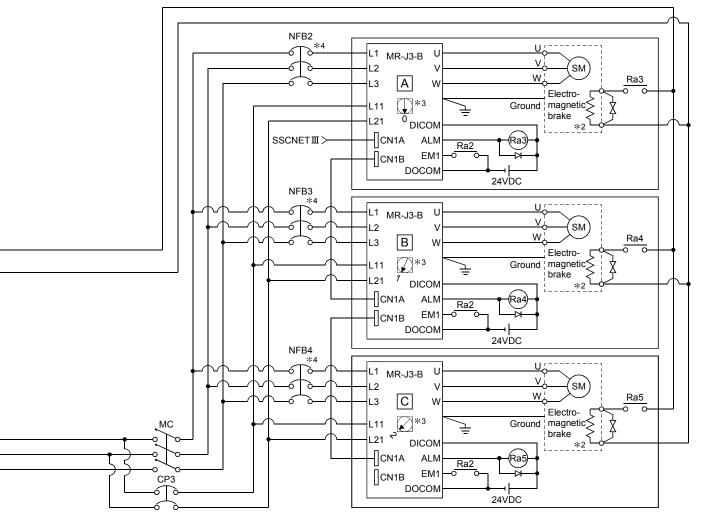
(Note-1): When the control power supply of servo amplifier is shut off, it is not possible to communicate with the servo amplifier after that. Example) When the control power supply L11/L21 of servo amplifier in above B figure is shut off, it is also not possible to communicate with the servo amplifier Cl.
