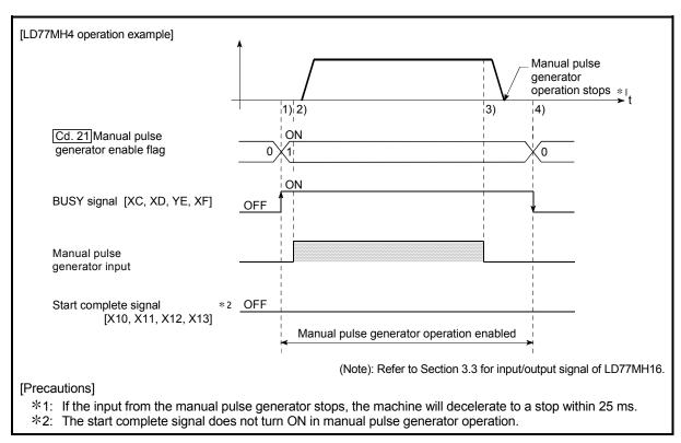
Fig. 11.16 Manual pulse generator operation
