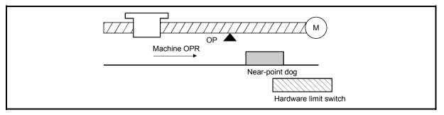
(6) When the zero signal is detected again during deceleration (4) of Fig. 8.12) with detection of zero signal, the operation stops at the zero signal detected lastly to complete the OPR.
