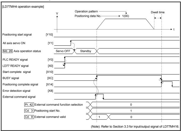
Fig. 6.11 Time chart for starting with external start signal
