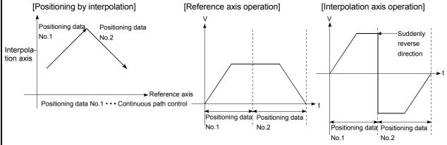
(2) When a "0" is set in the " Da.6 Positioning address/movement amount" of the continuous path control positioning data, the command speed of about 2 ms is reduced to 0.
