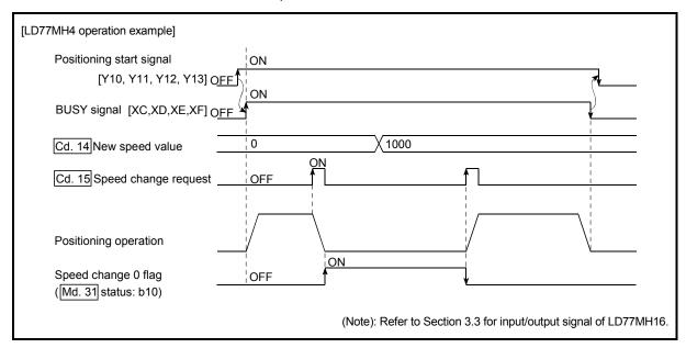
Fig. 13.25 Speed change at new speed value "0"
