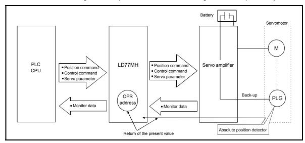
Fig. 13.35 Configuration of absolute position system
