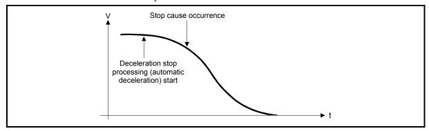
Fig. 13.52 Deceleration curve continuation operation (for position control or S-curve acceleration/deceleration processing)
