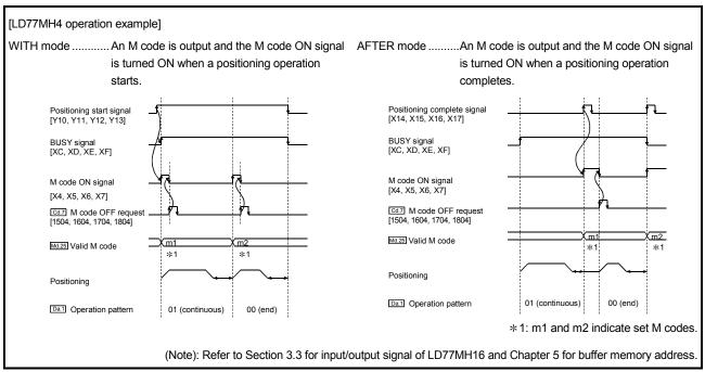
Note: If AFTER mode is used with speed control, an M code will not be output and the M code ON signal will not be turned ON.
