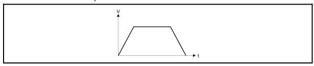
Fig. 13.45 Trapezoidal acceleration/deceleration processing method
