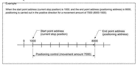
[When "1-axis linear control (ABS linear 1)" is set in positioning data No. 1 of axis 1.]
