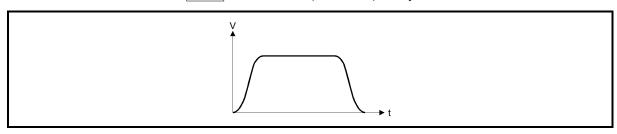
Fig. 13.46 S-curve acceleration/deceleration processing method
