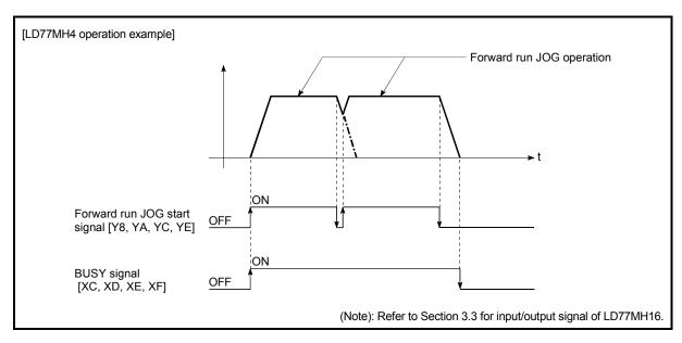
Fig. 11.9 Operation when the JOG start signal is turned ON during deceleration
