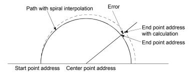
\*1: With circular interpolation control using the center point designation, the arc path calculated with the start point address and center point address and the end point address may deviate.
