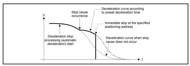
Fig. 13.51 Deceleration curve re-processing operation (for position control or S-curve acceleration/deceleration processing)
