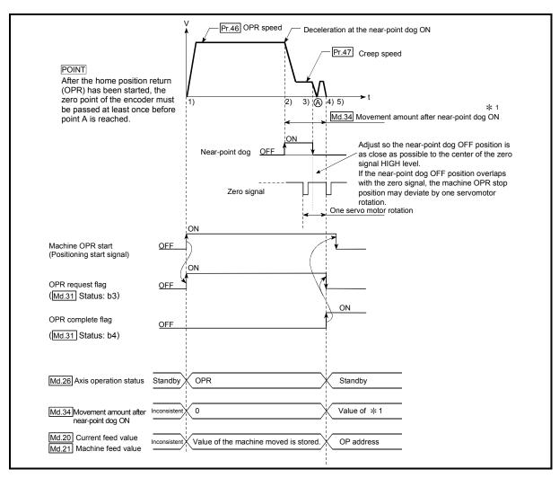
Fig. 8.3 Near-point dog method machine OPR
