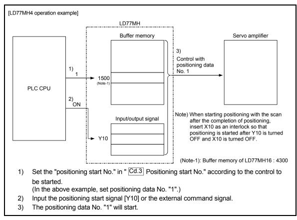
Fig. 6.2 Procedures for starting control (for axis 1)
