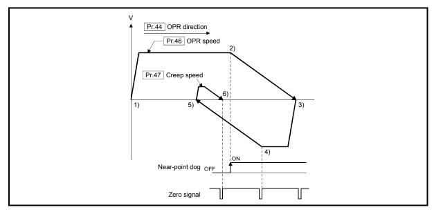
Fig. 8.12 Operation when the zero signal is detected again during deceleration with detection of zero signal
