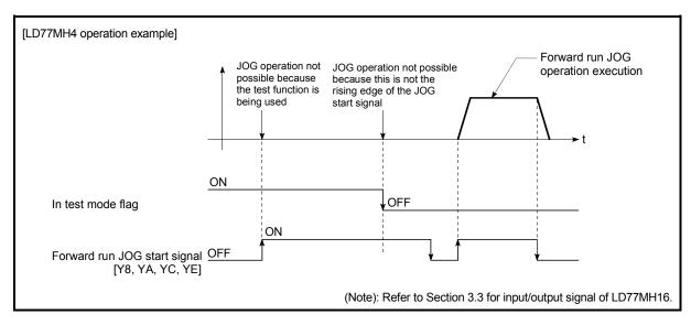
Fig. 11.10 Operation when the JOG start signal is turned ON while the test function is used
