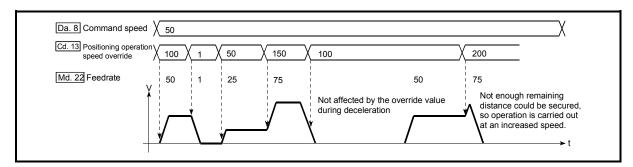
Fig. 13.28 Override function operation
