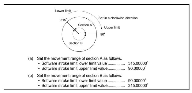
Fig. 13.16 Software stroke limit when the control unit is "degree"
