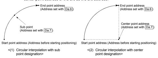
When not carrying out circular interpolation control, the value set in " Da.7 Arc address" will be invalid.
