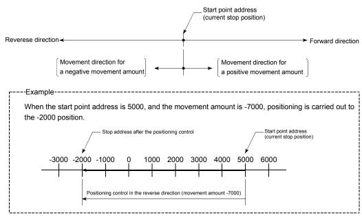
[When "1-axis linear control (INC linear 1)" is set in positioning data No. 1 of axis 1]
