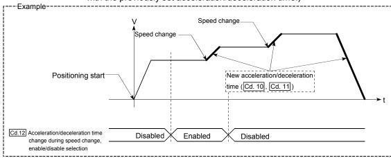
(4) If the "new acceleration/deceleration time" is set to "0" and the speed is changed after the "new acceleration/deceleration time" is validated, the operation will be controlled with the previous "new acceleration/deceleration time".
