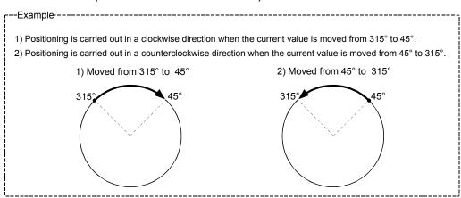
To designate the positioning direction (not carrying out the shortcut control), the shortcut control is invalidated and positioning in a designated direction is carried out by the "Cd.40 ABS direction in degrees".
