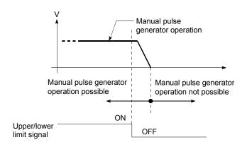
Manual pulse generator operation timing and processing time The following drawing shows details of the manual pulse generator operation timing and processing time.
