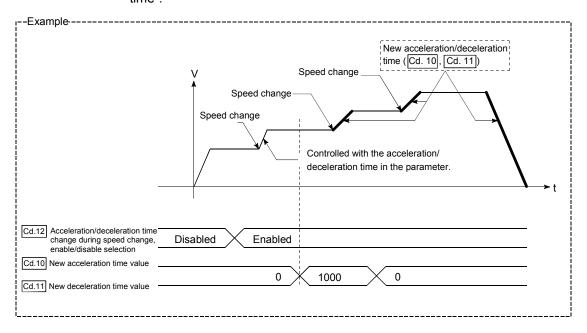
(5) The acceleration/deceleration change function cannot be used during speed control mode and torque control mode. Refer to Section 12.1"Speed-torque control" for the acceleration/deceleration processing during speed control mode.
