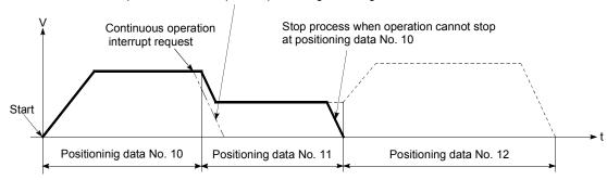
(4) When operation is not performed (BUSY signal is OFF), the interrupt request during continuous operation is not accepted. It is cleared to 0 at a start or restart.
