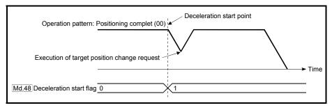
(6) When the movement direction is reversed by a target position change, the deceleration start flag turns ON.
