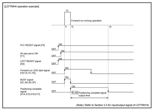
Fig. 11.11 Inching operation
