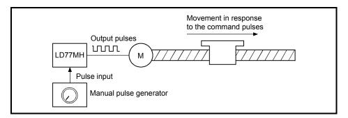
Fig. 11.3 Manual pulse generator control
