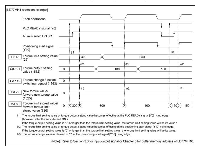
Fig. 13.11 Torque limit function operation
