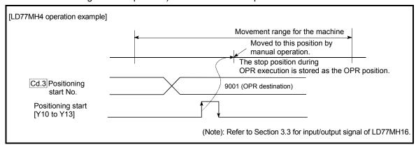
Fig. 13.36 Operation of the OPR execution
