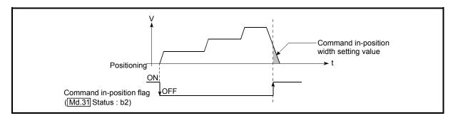
Fig. 13.43 Command in-position operation
