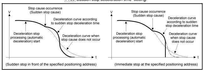
Fig. 13.53 Sudden stop operation (for position control or S-curve acceleration/deceleration processing)
