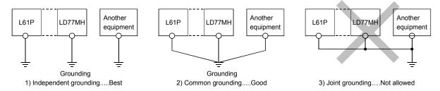
(c) For grounding a cable, use the cable of AWG16 to AWG20 (1.31 to 0.517mm<sup>2</sup>).
