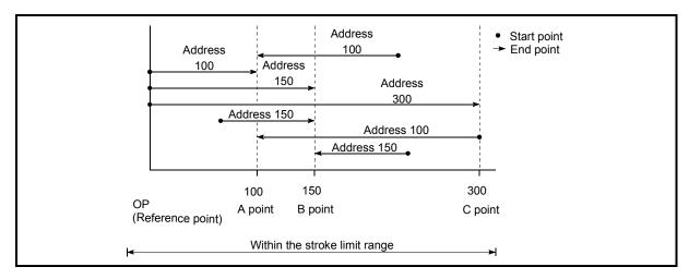
Fig. 9.6 Absolute system positioning
