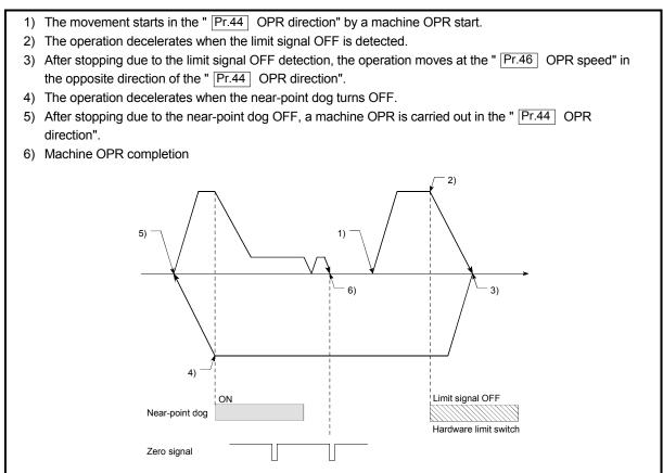
Fig. 13.1 OPR retry operation by limit signal detection
