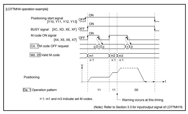
Fig. 13.42 Warning due to an M code ON signal during continuous path control
