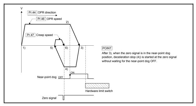
Fig. 8.10 Scale origin signal detection method machine OPR
