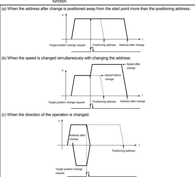
Fig. 13.33 Target position change operation
