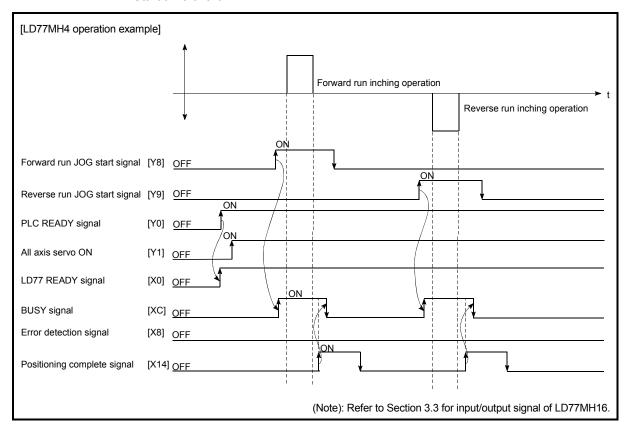
Fig. 11.13 Inching operation start time chart
