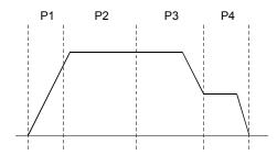
[When the movement amount is small during automatic deceleration]
