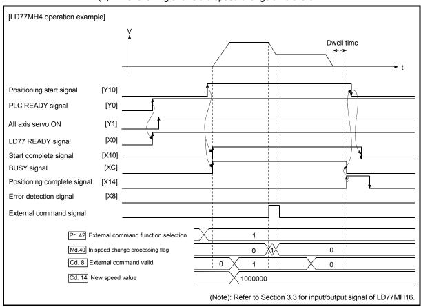
Fig. 13.27 Time chart for changing the speed using an external command signal
