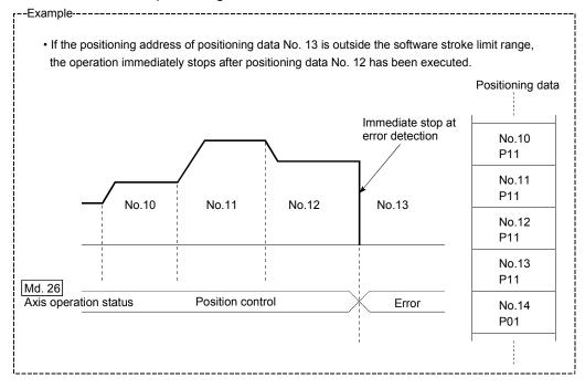
(5) During simultaneous start, a stroke limit check is carried out for the current values of every axis to be started. Every axis will not start if an error occurs, even if it only occurs in one axis.
