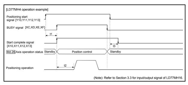
Fig. 8.14 Operation timing and processing time of fast OPR
