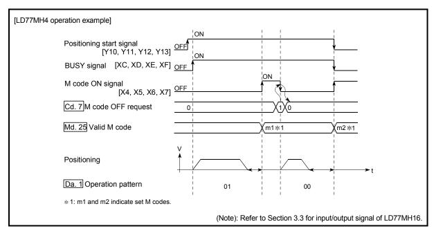
Fig. 13.41 M code ON/OFF timing (AFTER mode)
