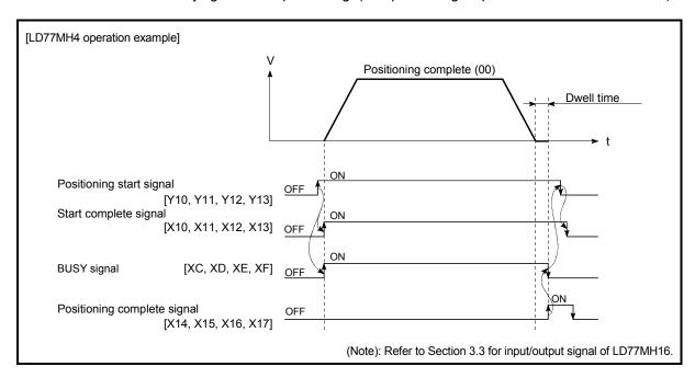
Fig. 9.1 Operation during independent positioning control
