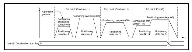
Fig. 13.50 Operation of deceleration start flag at block start
