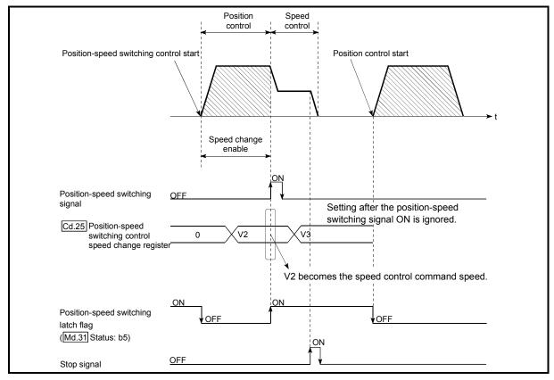
Fig. 9.20 Speed control speed change timing
