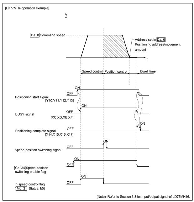
Fig. 9.16 Speed-position switching control (ABS mode) operation timing
