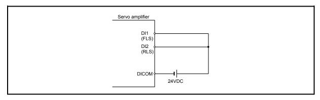
Fig. 13.19 Wiring when not using the hardware stroke limit function (When " Pr.22 Input signal logic selection" is the initial value)
