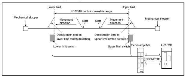
Fig. 13.17 Hardware stroke limit function operation
