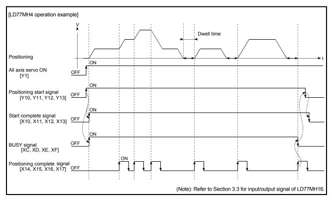
Fig. 6.3 ON/OFF timing of each signal at start of positioning
