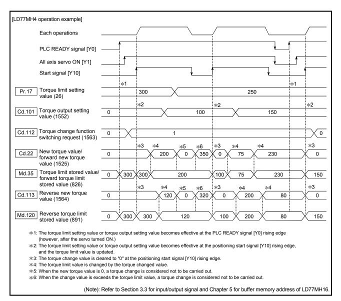
Fig. 13.32 Torque change operation (forward/reverse new torque value: individual setting) (Axis 1)
