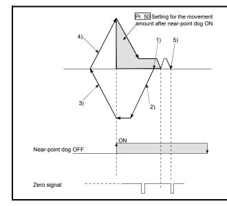
[Operation when a machine OPR is started at the near-point dog ON position]
