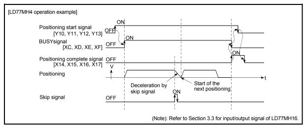
Fig. 13.39 Operation when a skip signal is input during positioning control
