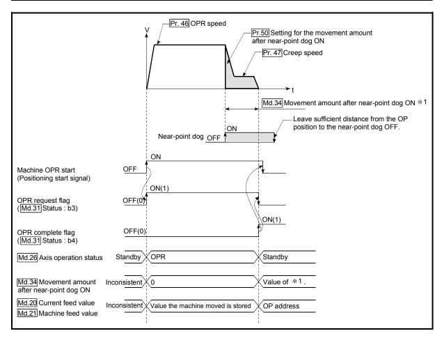
Fig. 8.7 Count method 2) machine OPR
