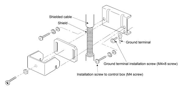
Using the AD75CK, you can tie four cables of about 7mm outside diameter together for grounding.
