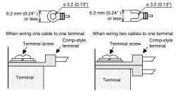
RAV1.25-3 (conforming to JIS C2805) V1.25-3 (manufactured by JST Mfg. Co., Ltd.) style terminal 1.25-3 and TG1.25-3 (manufactured by NICHIFU Co., Ltd.) Applicable wire size 0.3 to 1.25 mm<sup>2</sup>
