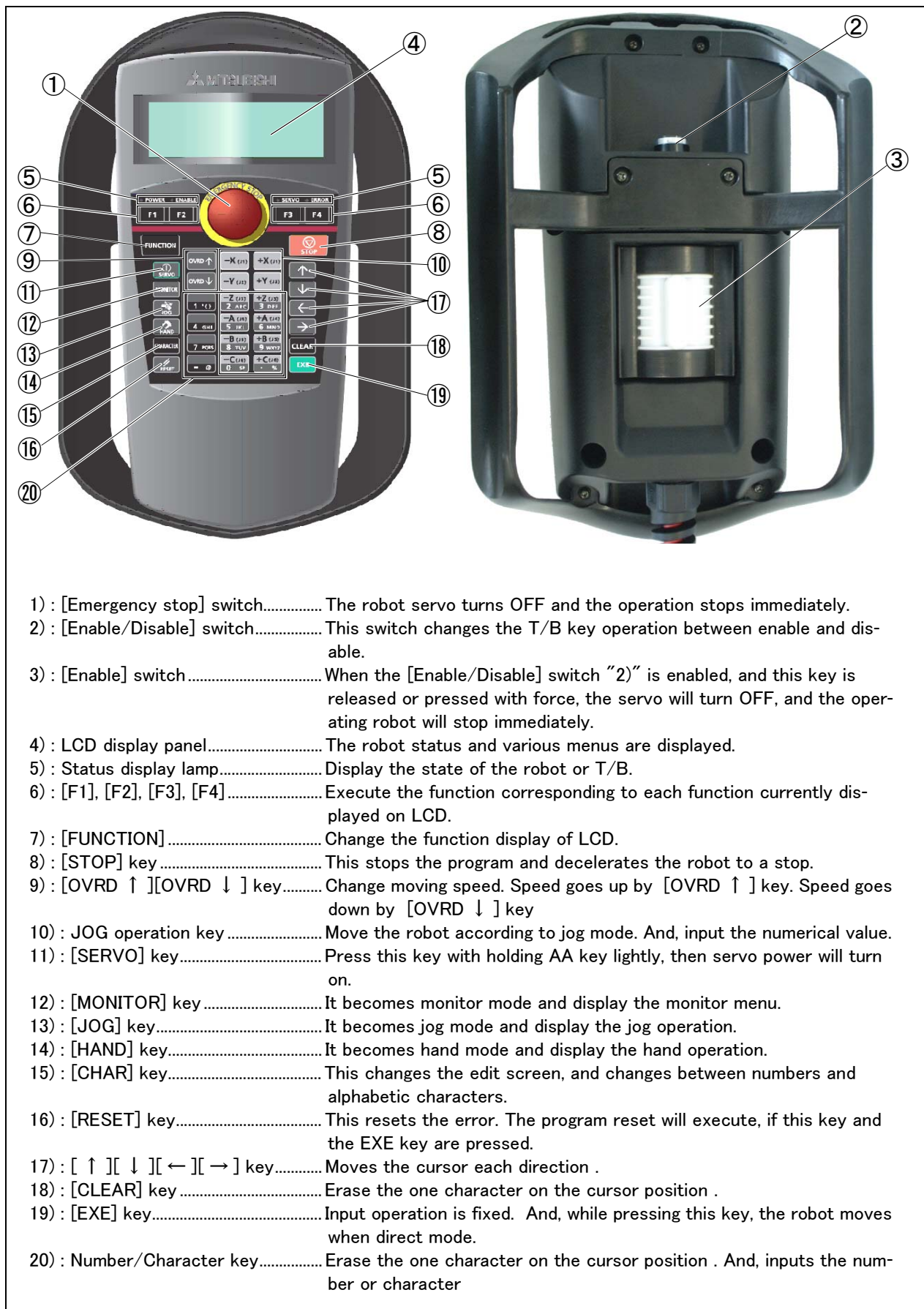
Fig.3-41 : Teaching pendant key layout and main functions
