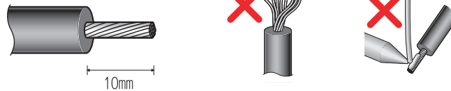
Cable sheath stripping length
