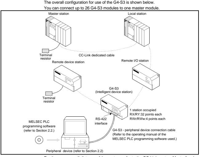
For the max. overall distance of the system, refer to the CC-Link system Master/local module user's manual.
