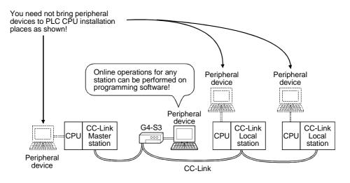
(2) Various peripheral devices can be connected.
