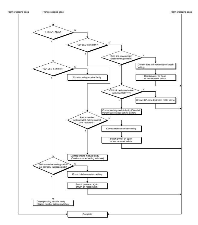
\*1: Check for short circuit, reverse connection, wire breakage, no terminal resistor, improper FG connection, improper overall distance and improper interstation distance.
