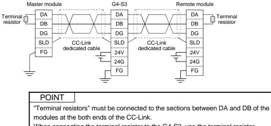
When connecting the terminal resistor to the G4-S3, use the terminal resistor supplied with the Master module.
