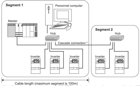
\* Up to four units are connectable when the 10 BASE-T is used and up to two units are connectable when 100 BASE-TX is used.
