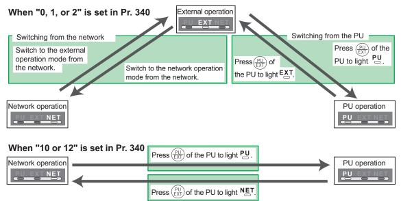
For the switching method from the external terminal, refer to *the inverter manual (applied)*. Refer to *page 65* for a switching method from the network.
