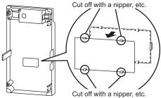
2)Fit the communication option LED display cover to the front of the inverter front cover and push it into until fixed with hooks.
